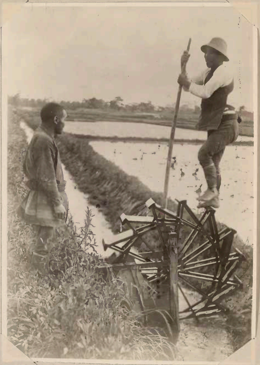
Fig. 9. Lifting water with a tread wheel in Japan
