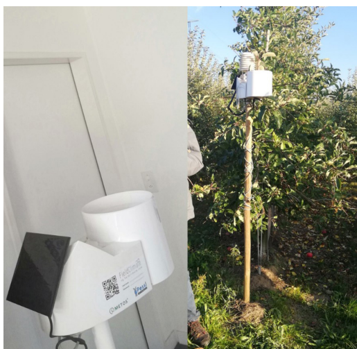
Figure 4: Example of a typical field sensor deployed in farming areas proposed within EUXDAT project. The sensor shown is an iMETOS 3.3 data logger developed by Pessl Instruments GmbH.
