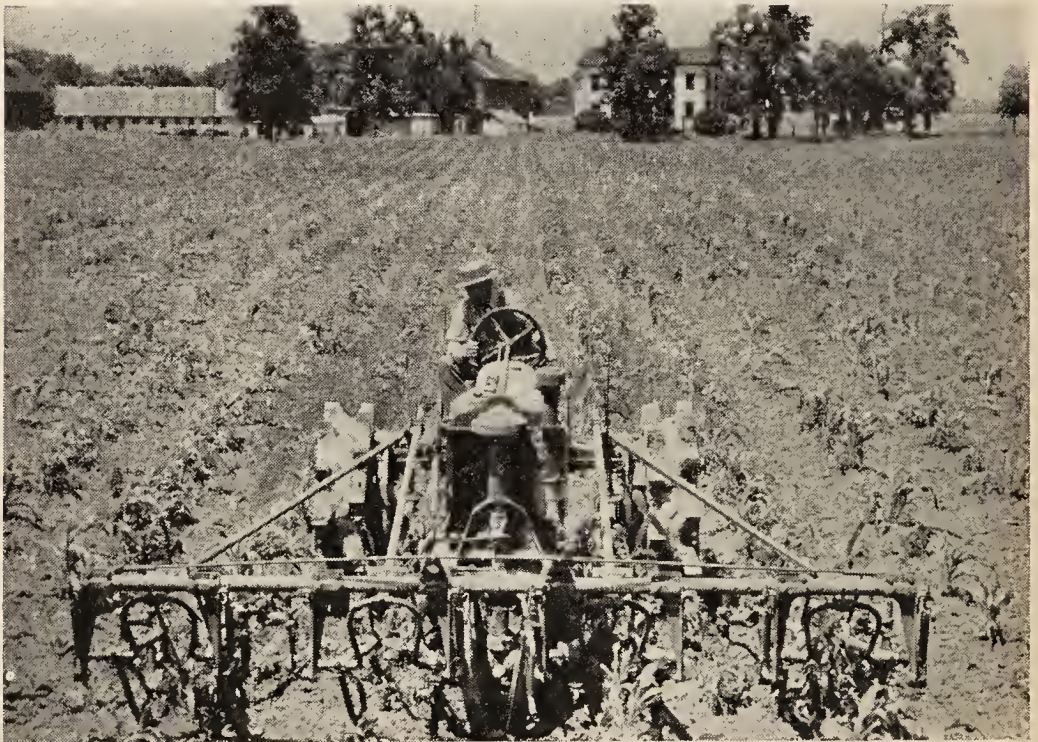
Figure 50. The use of tractor-powered cultivators has expanded rapidly with the increased use of general-purpose tractors. This is a four-row cultivator in a Minnesota cornfield (Bureau of Agricultural Economics.)
