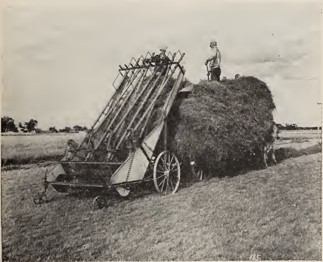
Figure 51. When a hay loader is used for loading, and a hay fork or slings are used for unloading, a crew of two men, one boy, and two horses can usually load, haul, and store about ten tons of hay in a day. (Bureau of Agricultural Economics.)
