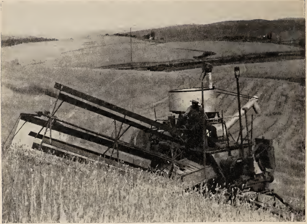
Figure 55. A modern grain combine that is especially adapted to grain harvest in hilly areas. On this machine the platform can be raised and lowered to conform to the slope of the land. (Bureau of Agricultural Economics.)
