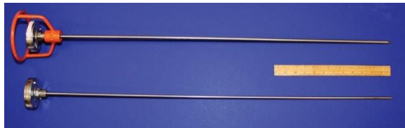
Photograph 1. Compost Thermometers are 3 to 4 feet Long
