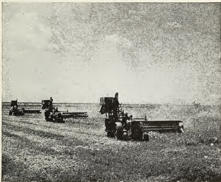
Figure 33. In the great wheat-producing areas of the United States, combines are the rule in harvesting the crop. These machines cut off the heads, thresh out the grain, and put it into sacks or storage bins, all in one operation. (U. S. D. A.)
