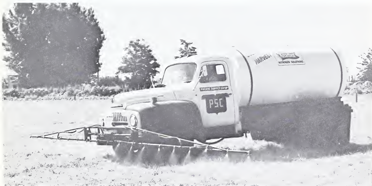
This truck is rigged with folding 32-foot booms for spraying both straight nitrogen and liquid mixed materials. The booms can be folded back when not in use.
