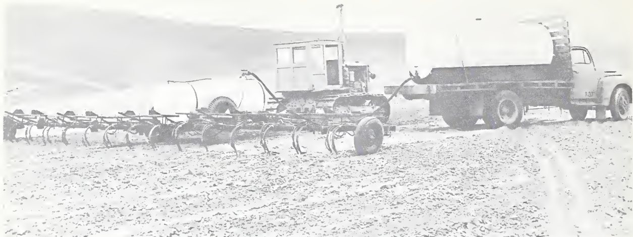
Aqua ammonia is transported to the farmer's field in nurse tanks on trucks or trailers and transferred to field applicators.
