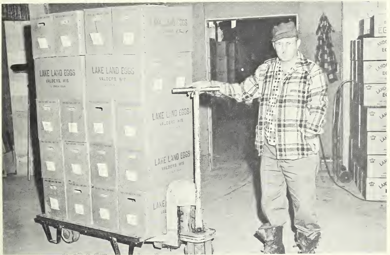
Skid and hydraulic hand truck. These eggs were brought into the egg receiving room on this truck from farm pick-up trucks.
