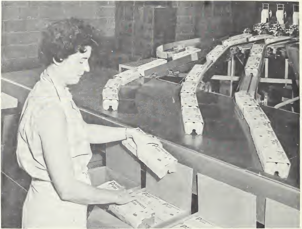
Packing cartoned eggs after cartons have been automatically filled, closed, sealed, and dated.
