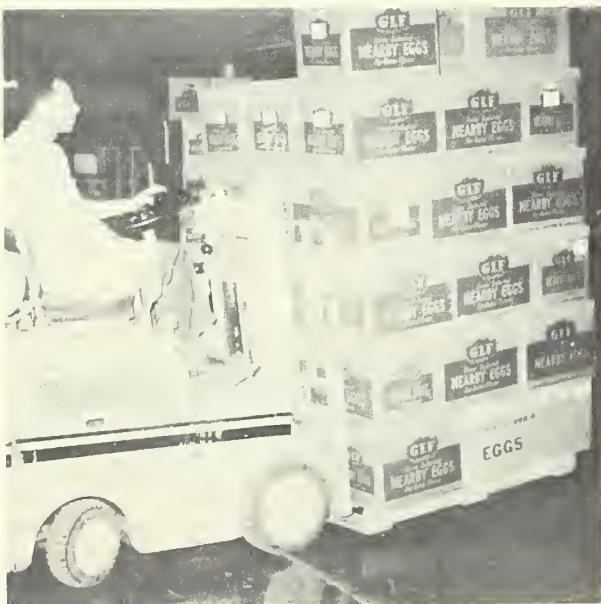
Skid and power lift truck. Through the use of these trucks in moving and loading eggs, cooperatives can save in labor costs.
