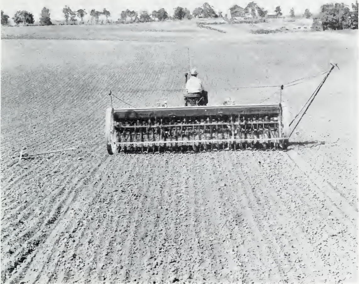
FIGURE 15.—Almost half of the drilling of small grains is done with tractor-drawn drills. These drills are used most extensively in the Great Plains, in the Pacific Coast States, and in the western Corn Belt. Under favorable conditions from 40 to 45 acres can be drilled a day with a 14-foot tractor-drawn drill. With the same size drill about 50 percent more work can be done with tractor power than with animal power.
