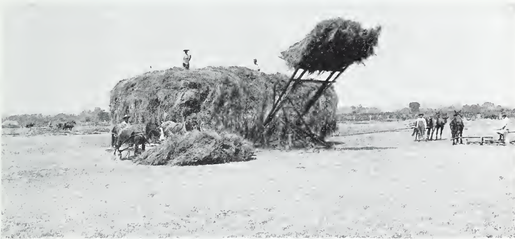
FIGURE 60.—Hay stackers are used largely in the western part of the country. When the haymaking crew is properly organized the use of hay stackers saves much time and eliminates much of the hard work. A fairly common stacking crew consists of five men and six horses. The crew includes two men and four horses operating two sweep rakes, one man and two horses operating the stacker, with two men stacking hay. After the hay is windrowed, about 30 tons of hay can be stacked in a 10-hour day with a crew of this size and with a stacker. When stackers are used, only about half the labor required by hand methods is necessary.
