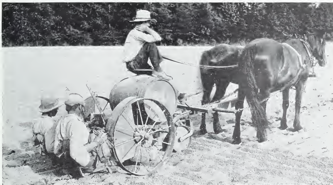
FIGURE 80.—Transplanting machines are used to a considerable extent in some tobacco areas. They can also be used for transplanting sweetpotatoes, cabbage, tomatoes, and other plants. When these machines are used, the plants are automatically watered when set. For pulling plants, hauling water, and for transplanting, from 20 to 30 hours of labor are used for each acre of tobacco plants set. Often some additional labor is needed for replanting.
