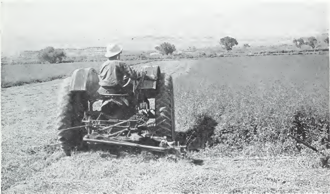
FIGURE 56.—Tractor-mounted mowers have come into fairly extensive use in some areas, especially on farms with large acreages of hay crops. Most of the hay acreage is cut in the summer months when care must be exercised to avoid the overheating of farm animals. This and the lack of animal power on many farms are the chief reasons for the increased use of tractor power for operating mowers. Tractor-mounted mowers usually cut a wider swath and are operated at higher speeds than animal-drawn mowers. With tractor power, mower performance is usually about 50 percent greater than for animal-drawn mowers of the same size.
