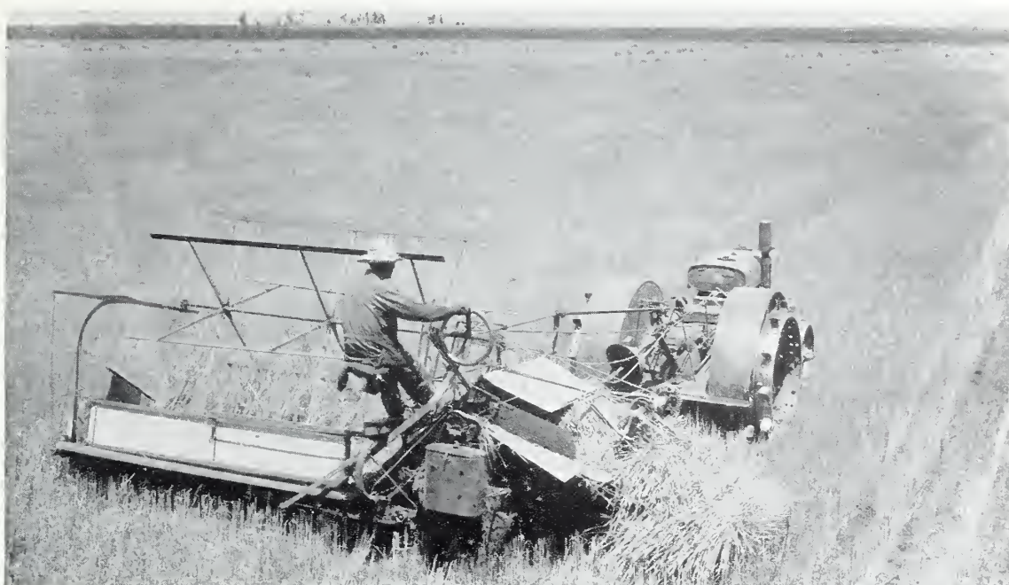
FIGURE 20.—Tractor power has come into extensive use for operating binders for small grain. Many of the tractor-drawn binders are the same binders that were previously operated with animal power, and they require a two-man crew. With the power binder, however, one man can operate both the tractor and the binder. In the major small-grain areas where the fields are large and level, tractor binders can cut about 3 acres a day for each foot of cutter bar. From 2 to 2.5 acres a day per foot of width is a fair achievement when the fields are of small size.
