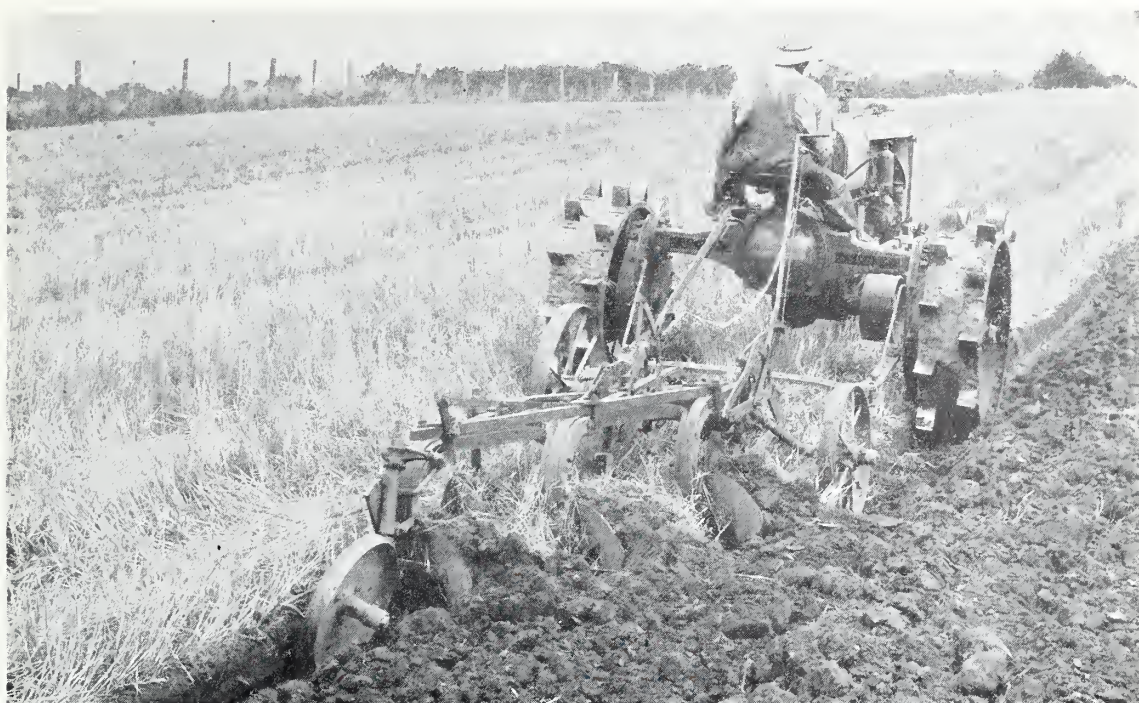
FIGURE 7.—Tractor power is extensively used for plowing, especially in the Great Plains, the western Corn Belt, the Rocky Mountain region and on the Pacific Coast. The three-bottom mouldboard plow is probably used most extensively in the Great Plains and the western Corn Belt. From 10 to 12 acres is a fair day's work for a tractor pulling three 14-inch-bottom plows.
