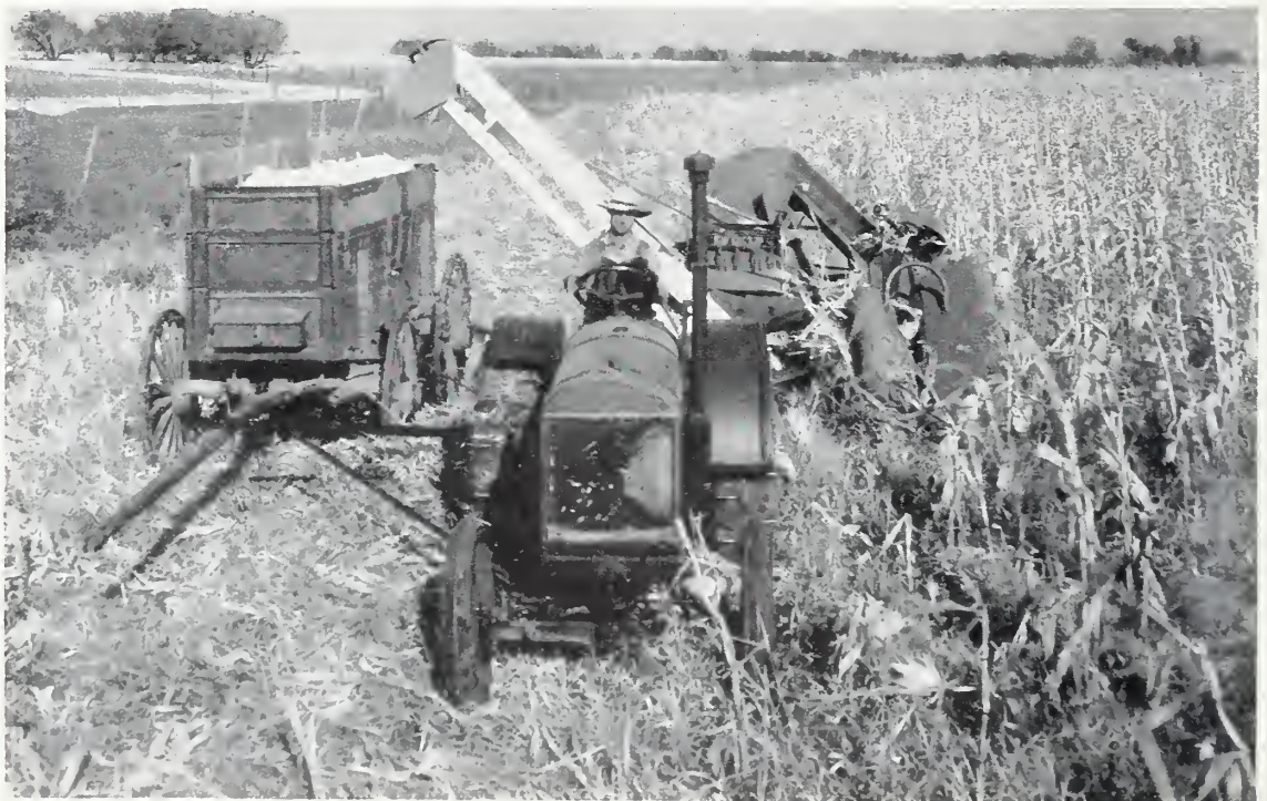
FIGURE 51.—Almost half of the acreage of corn harvested for grain in intensive corn-producing areas was harvested by mechanical pickers in 1938, and their use is increasing. With a two-row picker it usually takes from 2 to 3 hours of labor to husk and crib an acre of corn in the Corn Belt. From 6 to 8 hours of labor are needed to husk and crib an acre by hand methods.
