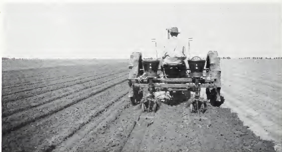
FIGURE 67.—Two-row lister planters are used for planting cotton in the western dry areas of Texas and Oklahoma. With a medium-sized tractor and a two-row cotton planter, a man usually plants about 18 acres of cotton in a 10-hour day.
