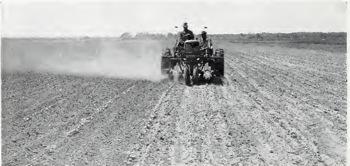
FIGURE 72.—Two-row tractor-drawn cultivators are used principally in areas where the cotton fields are level and where fairly large acreages of cotton are grown per farm. When the plants are small the cultivator is usually operated at a low speed to avoid covering the young plants. With a two-row tractor-drawn cultivator about 15 acres can be cultivated in a day in the early cultivations when the plants are small, and about 20 acres in the later cultivations.
