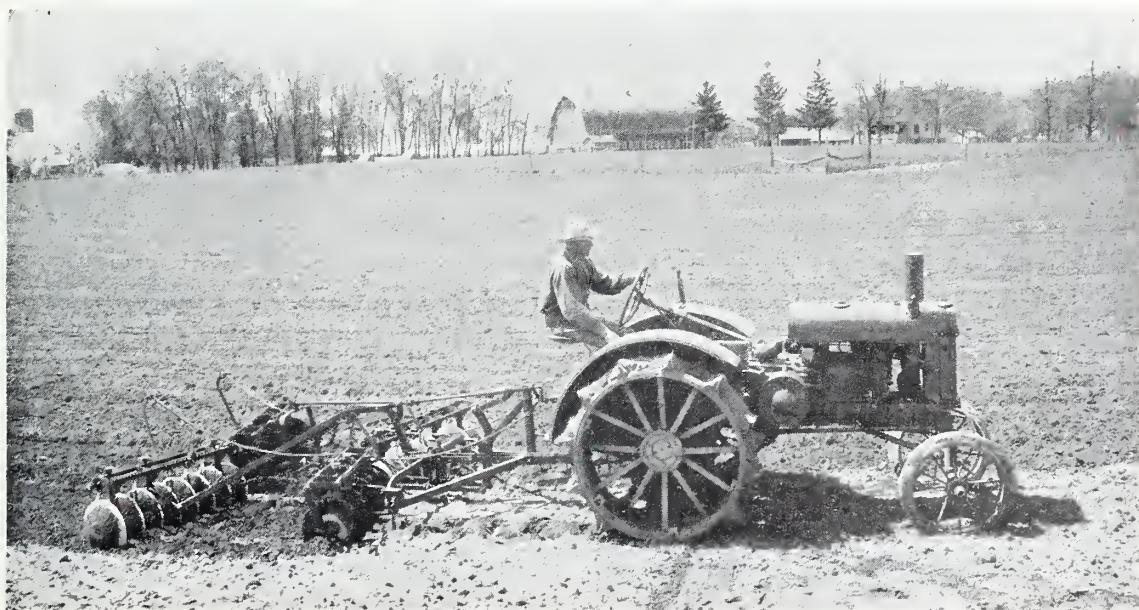
FIGURE 8.—Disk harrows are used extensively in connection with seedbed preparation, especially in areas where the soil type is relatively heavy. Disk harrows are also used extensively for cultivating orchards. Disking is heavy work and in most areas tractor-drawn disks are in common use. With a two-plow tractor and a 10-foot tandem disk or a 10-foot spring-tooth harrow, from 20 to 25 acres are usually covered in a 10-hour day.
