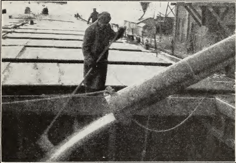
Figure 4.—Sampling cargo grain with a "pelican" at time of loading.
