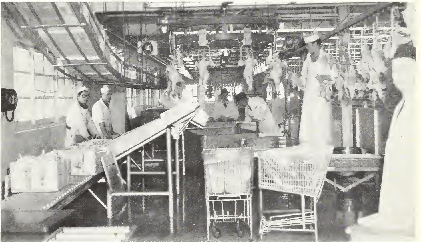
View of ice packing operation. Birds are transferred from chilling line to sizer and then to packing table.
