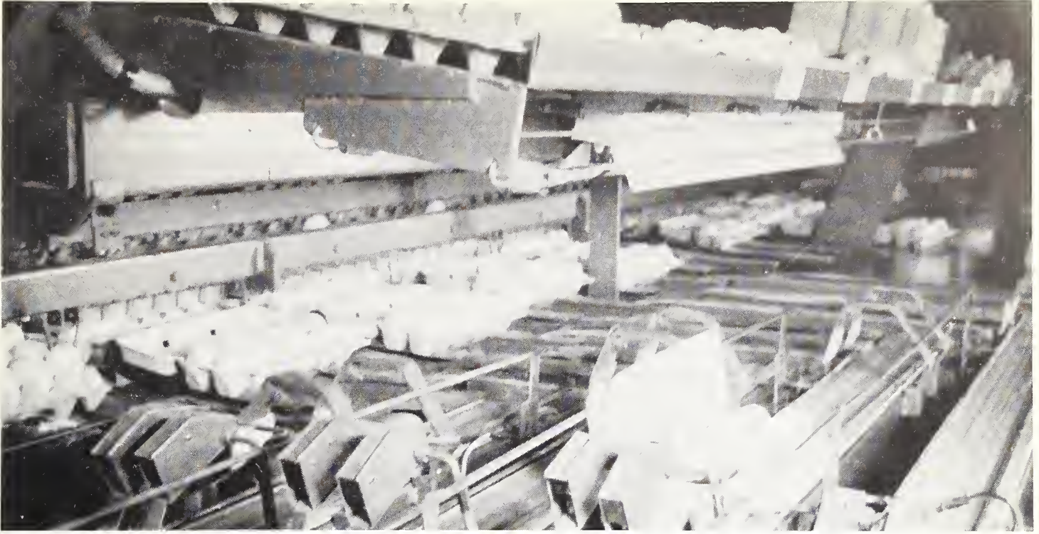
Closeup of the egg handling machine placing the eggs in fillers and cartons according to grade.
