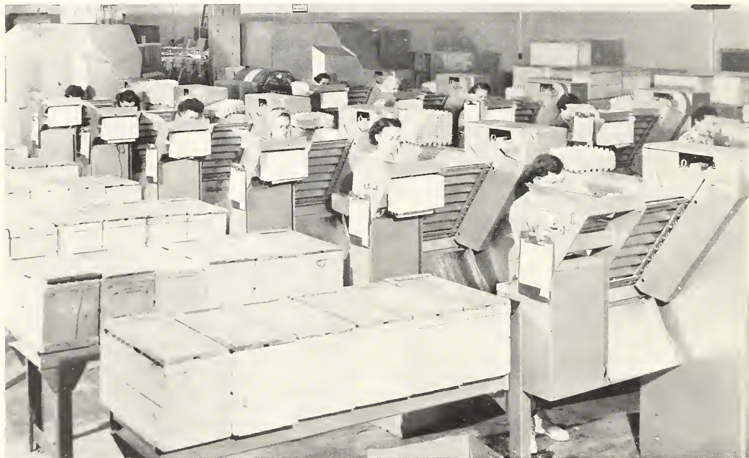
With newest make of equipment, after eggs are hand candled they are mechanically sized, shell processed, and placed in cartons or filler-flats ready for packing.
