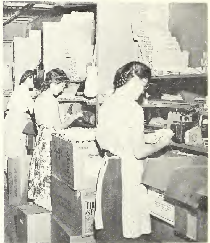
At most cooperatives in this study eggs are candled and cartoned in booths.
