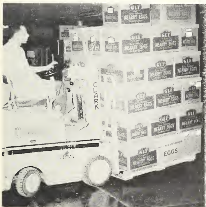
Power lift trucks are labor savers in moving and loading out eggs.
