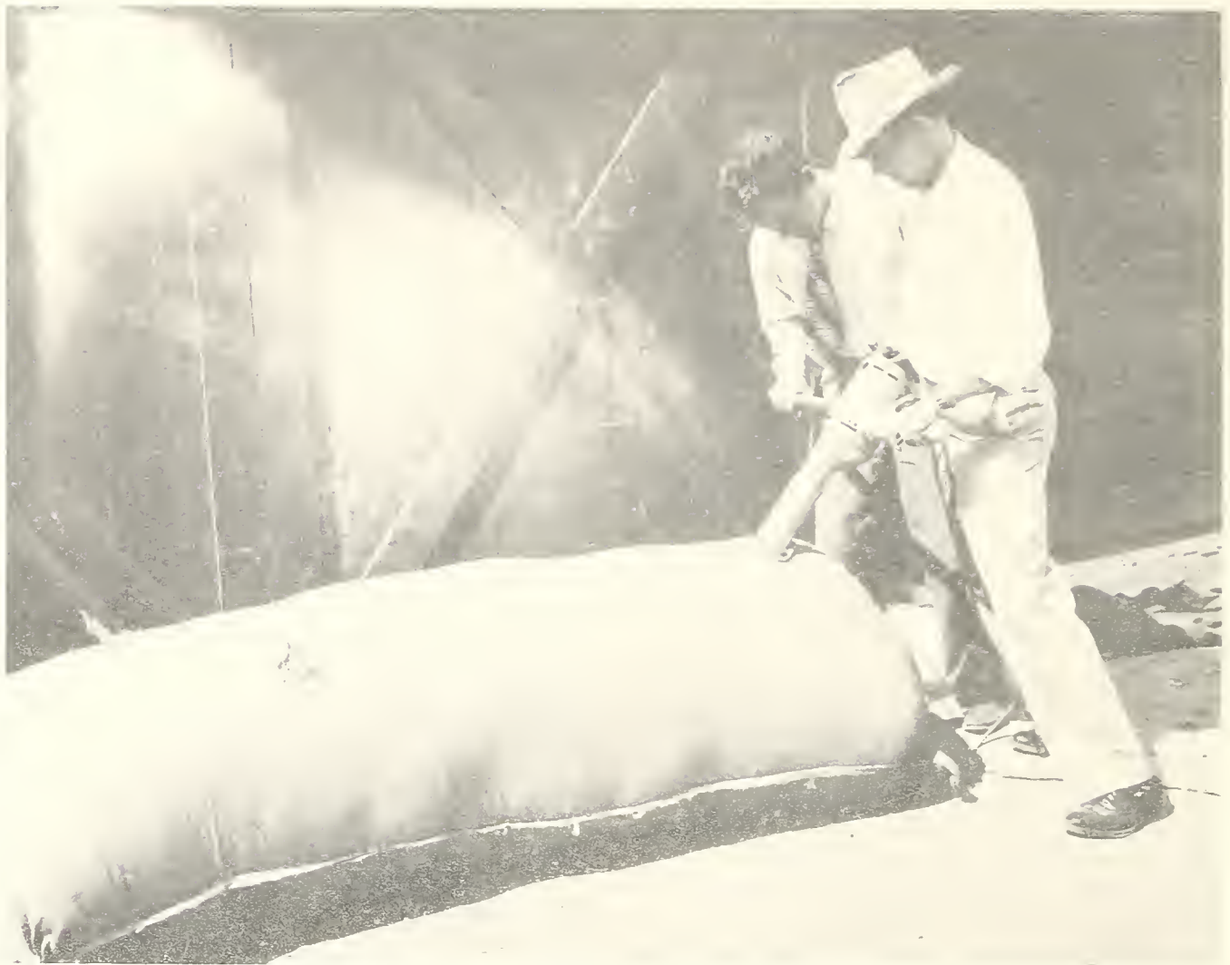
Drawing core samples with a 3 inch tube for laboratory testing of clean yield. Smaller tubes are becoming more popular.
