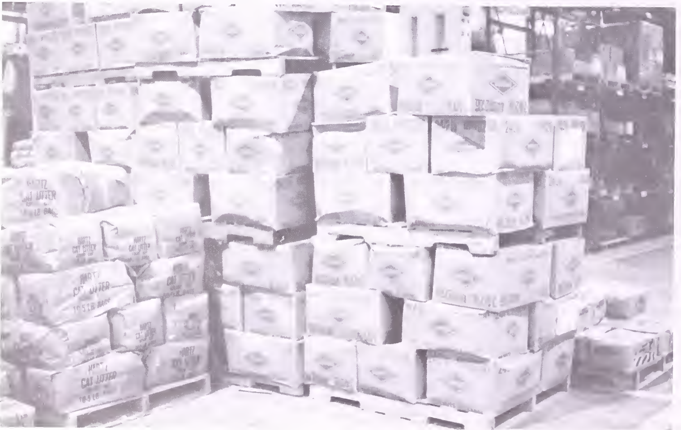
Figure 3.—Cases that have been crushed due to excessive stacking.
