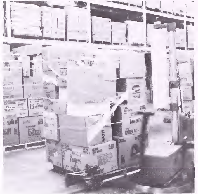
Figure 6.—A pallet load of mixed cases being shrink-wrapped by a robotic device.
