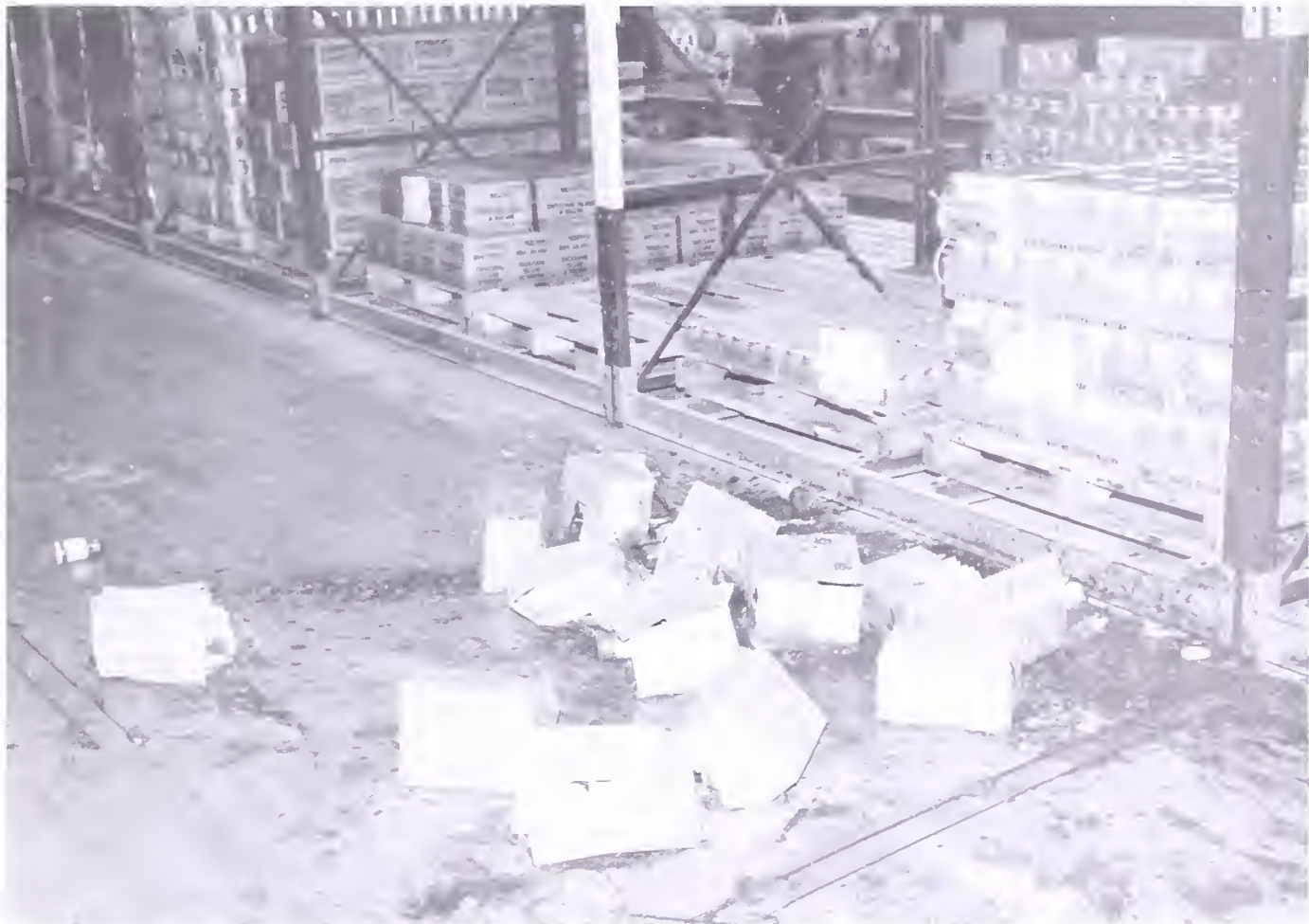
Figure 1.—Cases that have fallen from the upper rack because they were bumped during positioning in slot.
