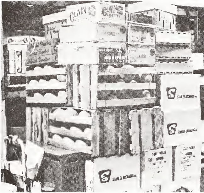
Figure 18.—A mixed produce load at the wholesale warehouse. Note wirebound crates of cantaloupes within load. They do not stack as well as the fiberboard containers of cantaloupes shown in the bottom two layers.
