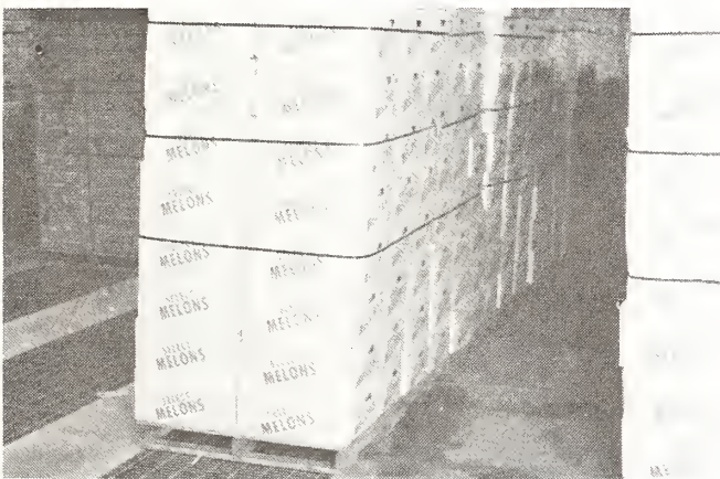
Figure 13.—Melons in fiberboard containers being forced-air cooled prior to loading on a highway trailer.
