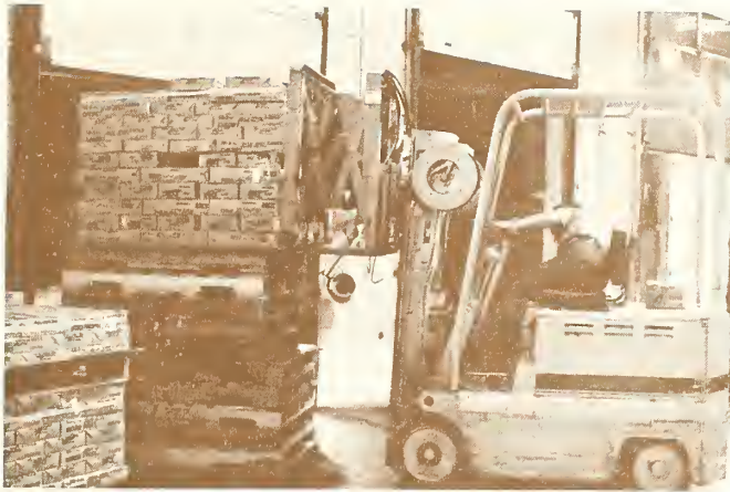
Figure 3.—A forklift truck, with a push-pull attachment, placing a slipsheet unit load on the top pallet.
