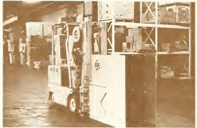
Figure 1.—Forklift truck with a clamp attachment used to transport unit loads from storage into trailer.
