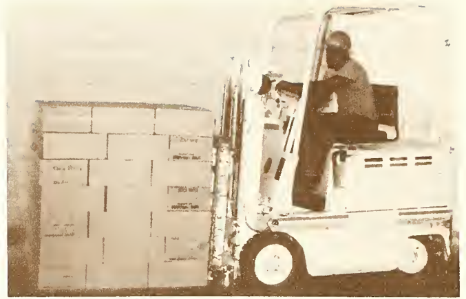
Figure 5.—A forklift truck with a push-pull attachment used to unload trailers having unitized slipsheet loads.
