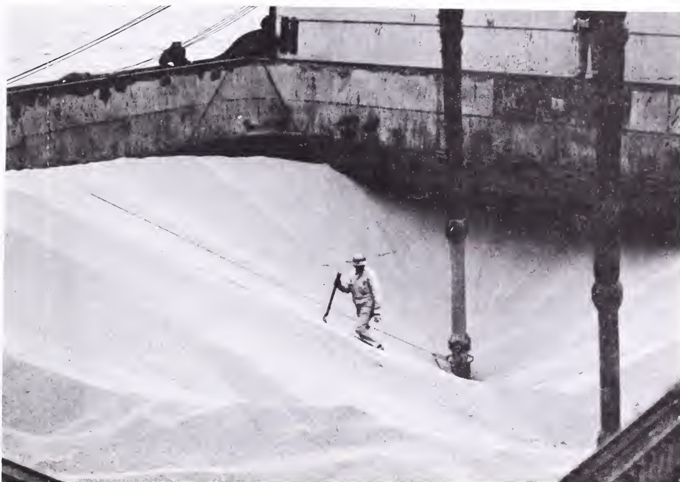
Figure 1.—Pneumatic unloading system, or "suckers," unloading soybean test shipment in Japan.
