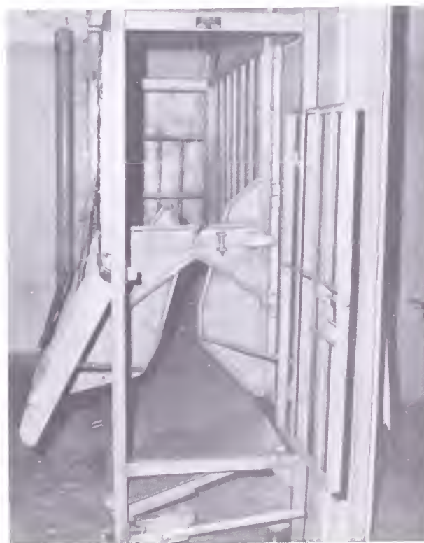
PN-4868 FIGURE 13.—Purchased stun pen with built-in head restrainer.
