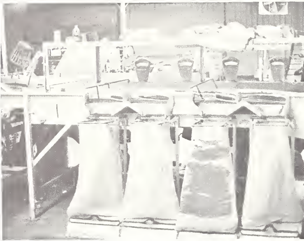
FIGURE 7.—Bagging stations for filling 100-pound burlap bags at a distribution table.
