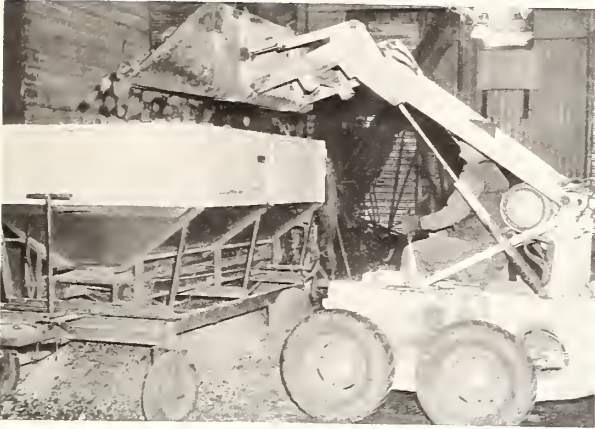
FIGURE 10.—Typical receiving hopper for a stationary location.
