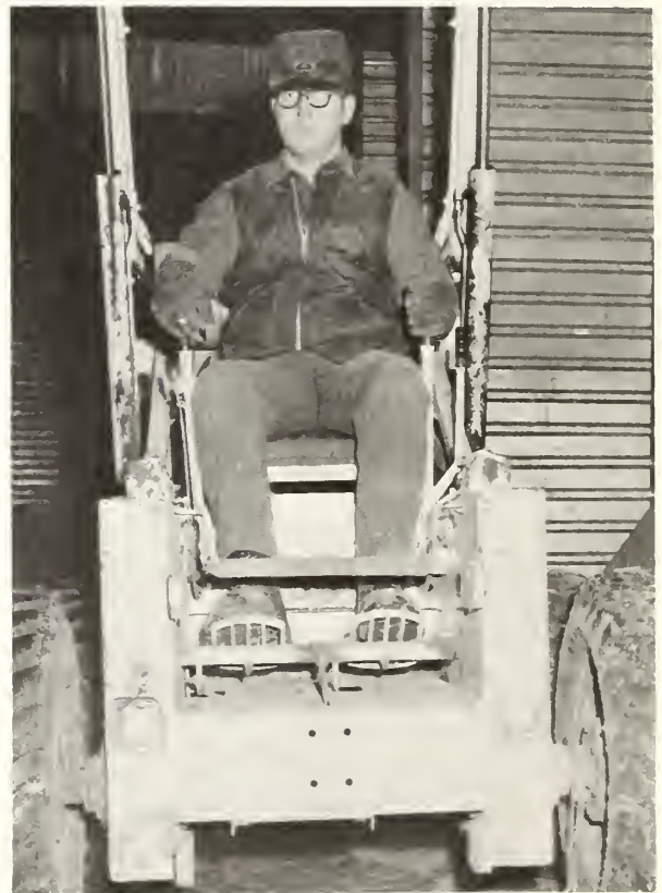
FIGURE 3.—Typical controls on a powered bulk scoop.
