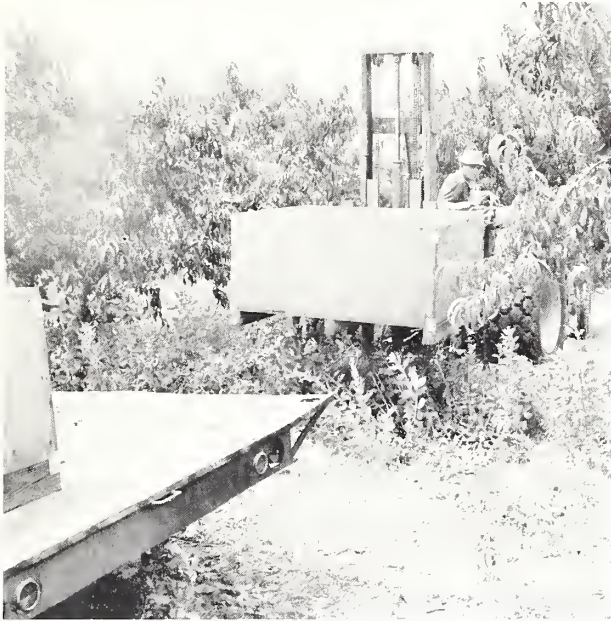
Figure 7.—The tractor-forklift transferring an empty pallet box from an orchard wagon to the ground.
