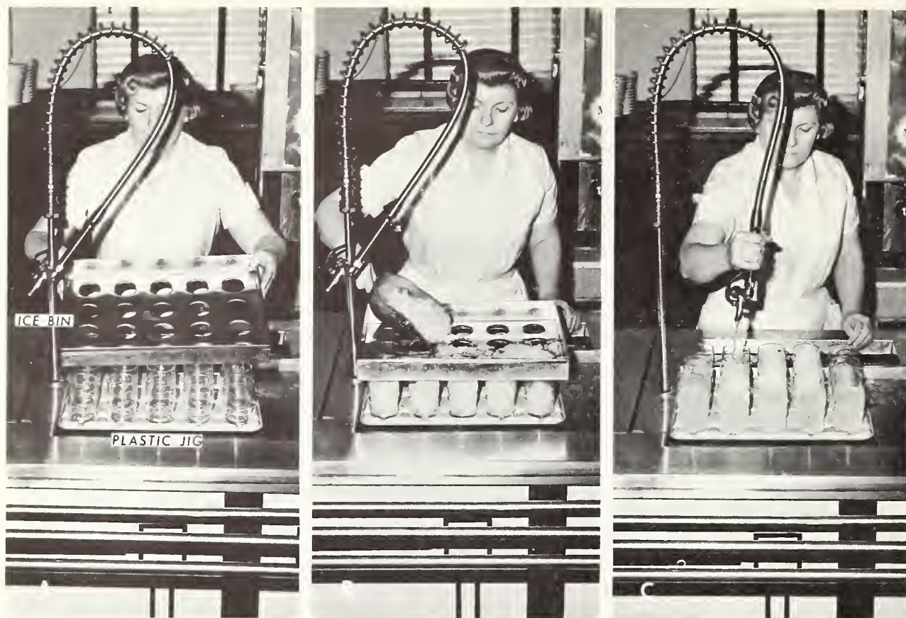
FIGURE 17.—Filling water glasses: A, Positioning ice bin over water glasses; B, placing ice in glasses using bin; C, filling glasses with water.
