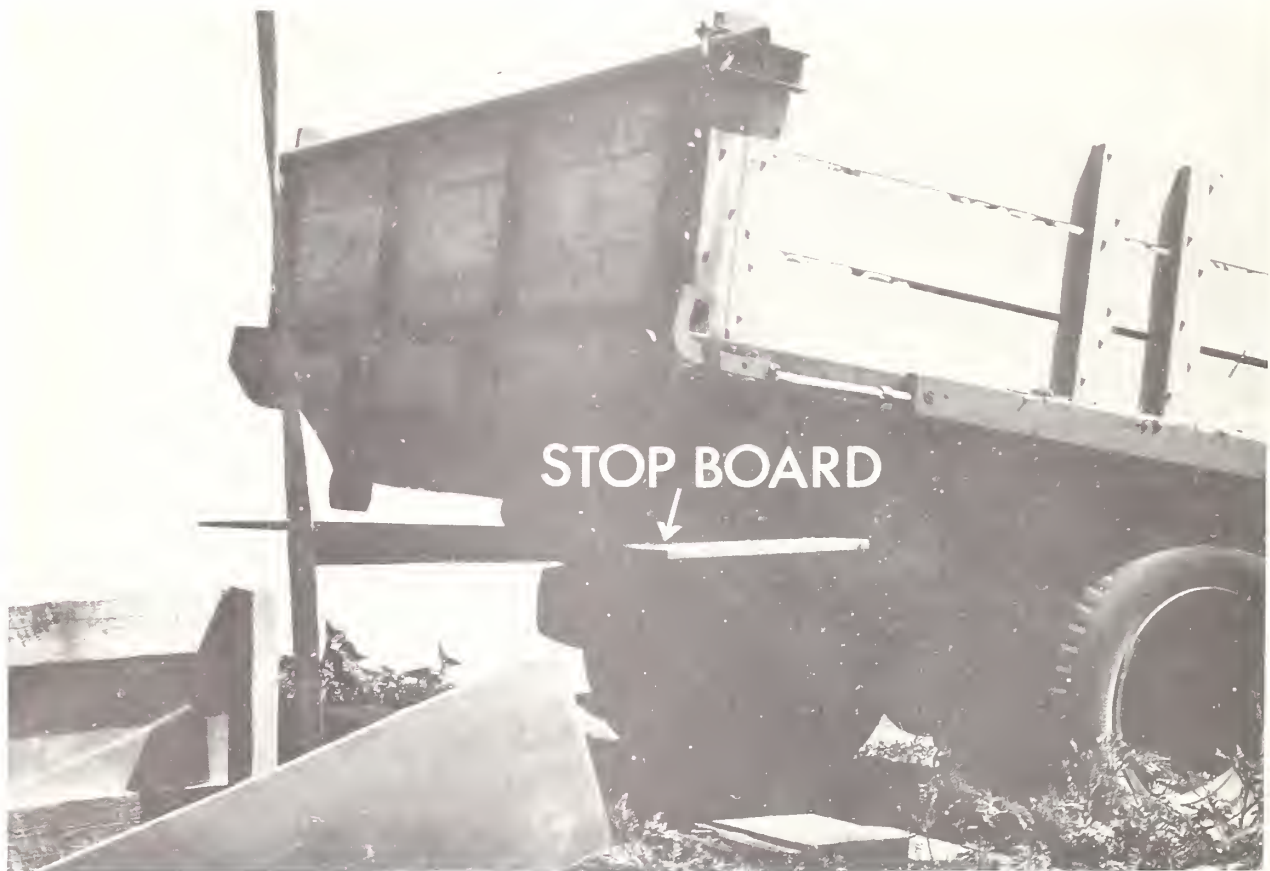
FIGURE 7.—The potato stopboard (below rear end of body) is shown in raised position as dump truck is backed into bin. During unloading the board is lowered.
