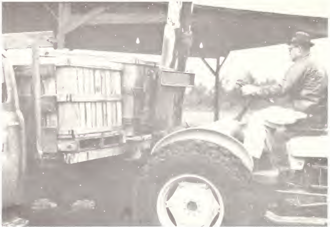
FIGURE 14.—Tractor forklift used in the experimental pallet box operation; view of removing a filled box from truck.
