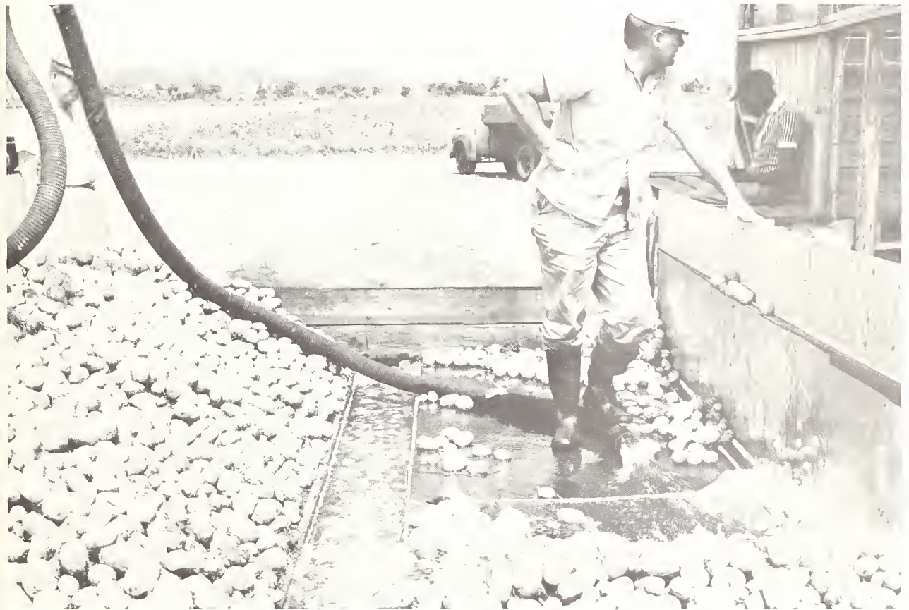
FIGURE 5.—Potatoes being washed into bin flume of the experimental bin with a water hose. Operator normally works from the front to the back along one side. Potatoes flow out at front of bin just behind hose.
