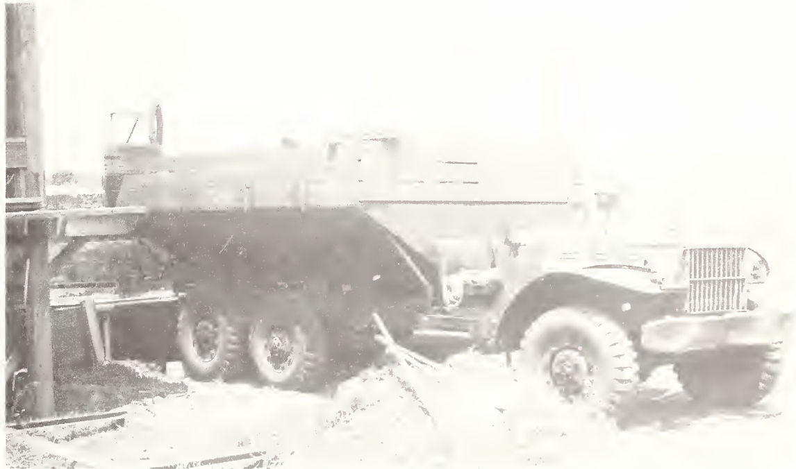
FIGURE 1.—A hopper-body truck. Potatoes are being unloaded into the flume. BN-26702
