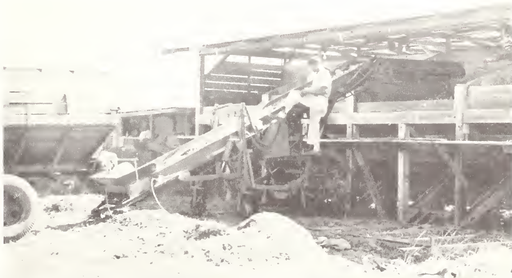
FIGURE 2.—Potatoes being unloaded from hopper-body truck into a sloping-bottom bin by a bin-loader conveyor. The bin loader moves on tracks parallel to a row of bins. BN-26703
