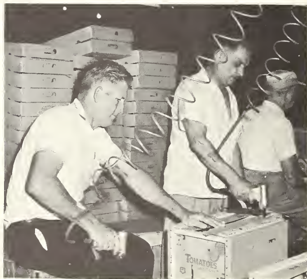
FIGURE 10.—Two-man crew closing nailed carton with pneumatic staple guns.
