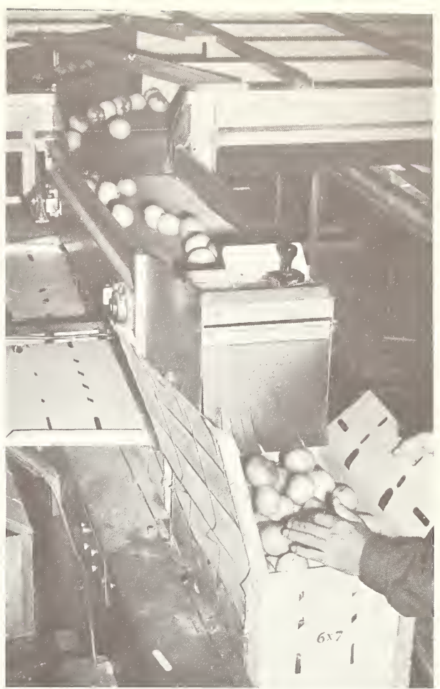
FIGURE 7.—A machine for filling 40-pound cartons and 60-pound wirebound boxes with tomatoes.
