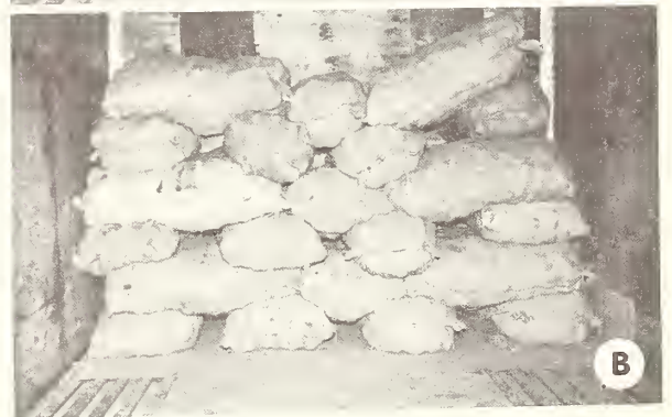
BN 23644, BN 23645 FIGURE 9. —Airflow pattern No. 5 for 100-pound burlap bags to provide air circulation channels; for use in either wide or narrow trailers. (A) First or header stack. (B) All subsequent stacks.
