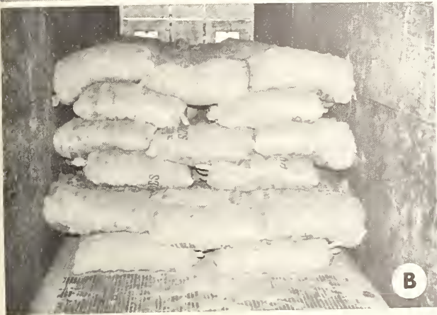
BN 23642, BN 23643 FIGURE 8. —Airflow pattern No. 4 for 100-pound burlap bags; for use in trailers with 2 inches of insulation or less. (A) First or header stack. (B) All subsequent stacks.
