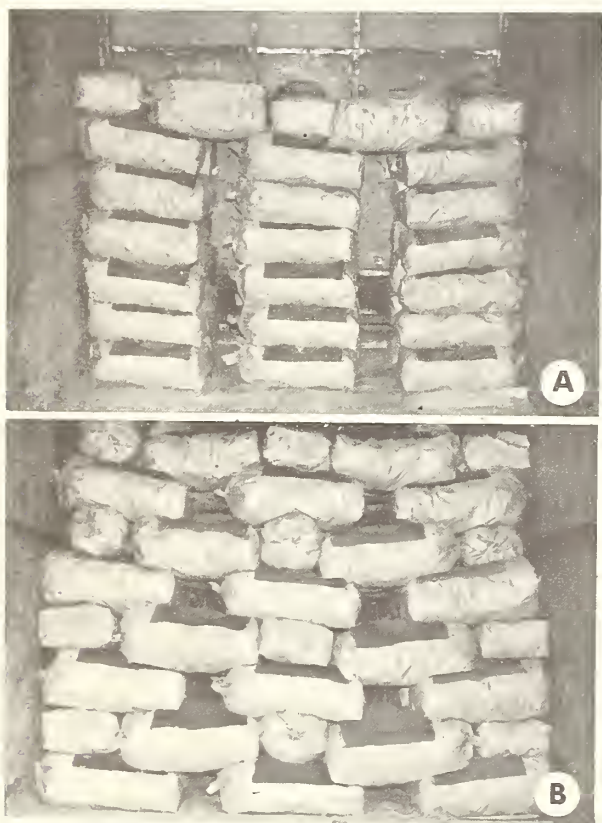
FIGURE 5.—Airflow pattern No. 1 using 50-pound paper sacks with twist-tie closure. (A) First or header stack. (B) All subsequent stacks.
