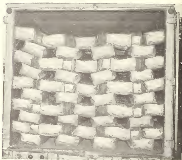
FIGURE 7.—Airflow pattern No. 3 using 50-pound tape-closure master paper sacks, each of which contains five 10-pound bags. This pattern is designed for use in wide trucks with header stack as shown in figure 6(A).
