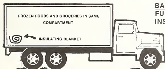
FIGURE 1.—Five basic systems for shipping mixed loads of frozen foods and groceries. (Detailed refrigeration equipment not shown for systems 3–5.)
