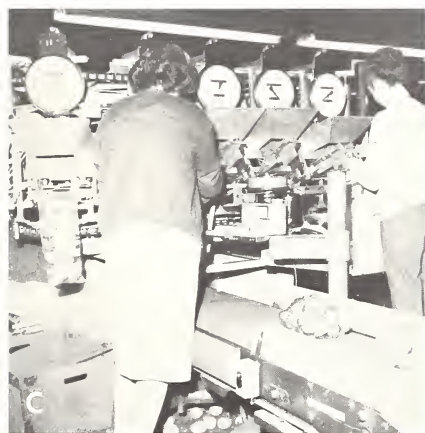
FIGURE 63.—Equipment for produce packaging at firm E; A, Hanging empty bags; B, checking for weight; C, bag closing; D, packout in baler bags.
