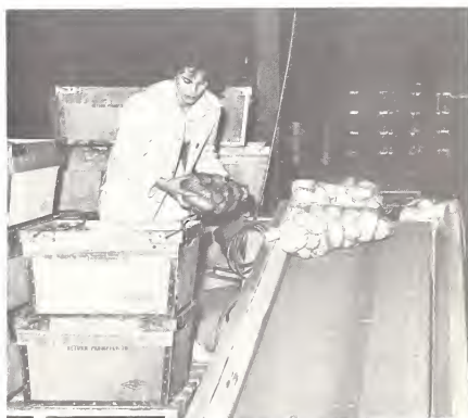
FIGURE 39.—A wooden stack-and-nest box for bagged produce.
