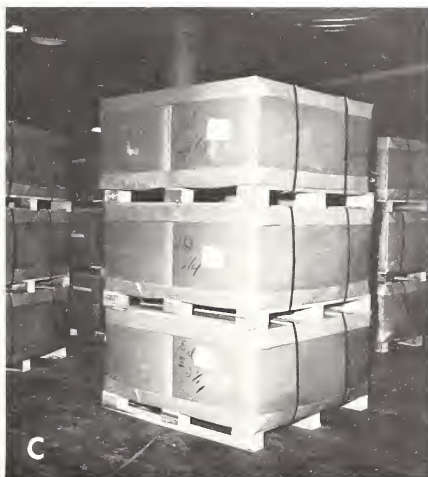
FIGURE 10.—Corrugated pallet containers: A , One-piece expendable box; B , double-wall box with 4-inch wide wooden slots between corrugated tubes at center of each side provide stacking strength and minimize bulging; C , two-cell box with identical top and base caps, a base pad, and lightweight reversible pallet base; D , one-cell triple wall container with the short side scored so the box will collapse for ease of handling.
