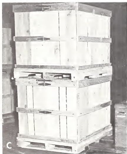
FIGURE 9.—Wooden pallet boxes. A , Wirebound with modified pallet base, the box is difficult to assemble and disassemble and is too long when collapsed. B , This 2-piece box collapses to 42- by 47-inches. A wooden flange holds the sides in place and 2 metal clips prevent the top from becoming disengaged from the base. C , Similar to box in B , its top is attached to the base with U-type metal clip. This box is used entirely for local haul of potatoes. D , This box has 4 plywood sides that are hinged together by 3 metal clips. The base is also attached to the top with metal clips.
