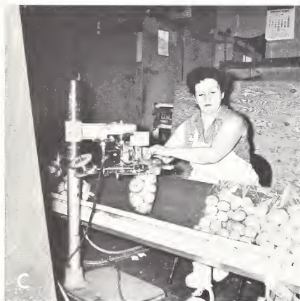
FIGURE 59.—Produce packaging equipment in firm B: A, Line feeding; B, bag filling; C, bag closing; and D, packout.
