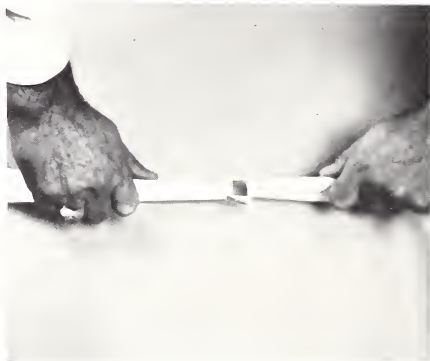
FIGURE 7.—Strapping the pallet container with a rayon cord. Pulling the two ends increases tension.
