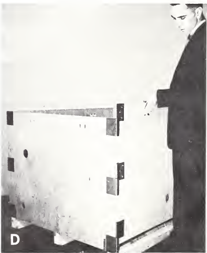
FIGURE 9.—Wooden pallet boxes. A , Wirebound with modified pallet base, the box is difficult to assemble and disassemble and is too long when collapsed. B , This 2-piece box collapses to 42- by 47-inches. A wooden flange holds the sides in place and 2 metal clips prevent the top from becoming disengaged from the base. C , Similar to box in B , its top is attached to the base with U-type metal clip. This box is used entirely for local haul of potatoes. D , This box has 4 plywood sides that are hinged together by 3 metal clips. The base is also attached to the top with metal clips.
