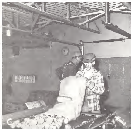
FIGURE 17.—Alternative methods of placing produce manually on a receiving belt: A, Into a floor chute; B, on belt from a raised platform; C, at belt height by two-man team; and D, from an adjustable lift platform.
