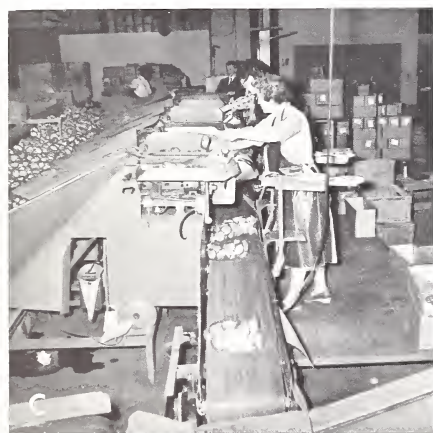
FIGURE 61.—The potato packaging line at firm D; A, Line feeding; B, hopper-type baggers; C, filling and closing; D, packout.
