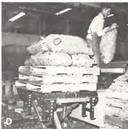
FIGURE 17.—Alternative methods of placing produce manually on a receiving belt: A, Into a floor chute; B, on belt from a raised platform; C, at belt height by two-man team; and D, from an adjustable lift platform.
