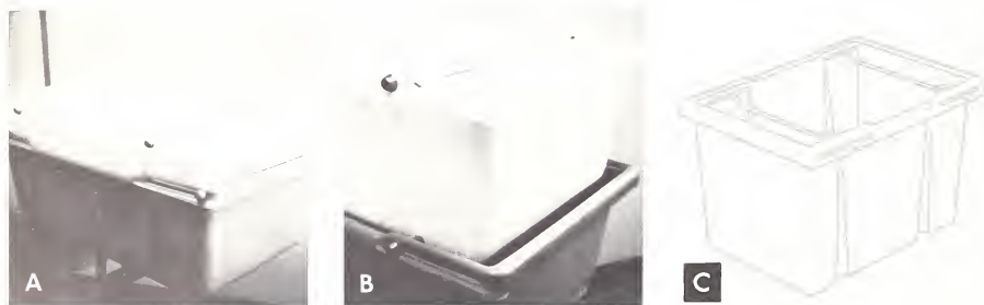
FIGURE 36.—A thermoplastic (polyethylene) container with sliding bails for stacking. (A) Bails are moved to recessed position in molded lip on bottom container for nesting and (B) toward the center for stacking. (C) perspective drawing.
