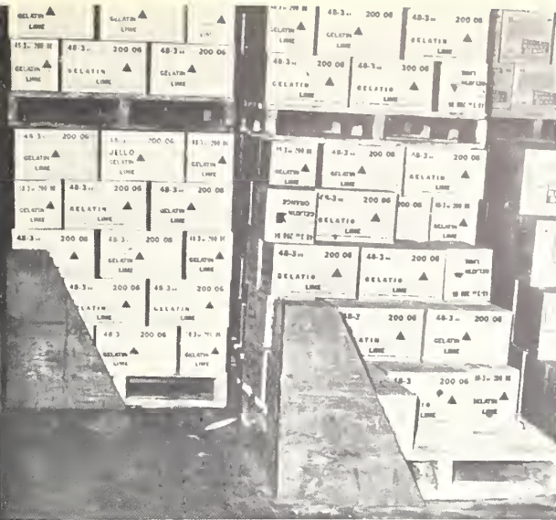
Figure 7.--(A) Metal guards used in one grocery warehouse for traffic corners; and (B) a closeup of the corner guards showing construction details.
