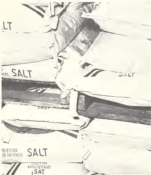
Figure 9.--Some examples of causes of warehouse damage: (A) Pallets of this type concentrate much weight on merchandise below; (B) insufficient clearances between pallets and columns; (C) insufficient clearance between pallets; and (D) forklift damage.
