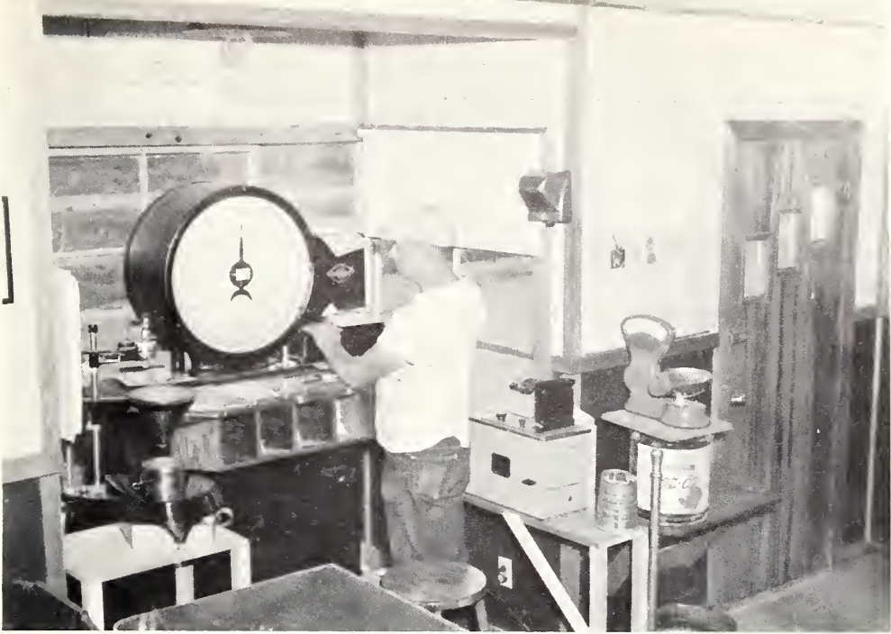
Figure 40. --Arrangement of equipment in the scale house when one man weighs trucks and determines the test weight and moisture content of grain. The moisture test equipment is at the right of the scale dial and the test weight equipment is at the left. The operator is placing a ticket in the scale printing mechanism.
