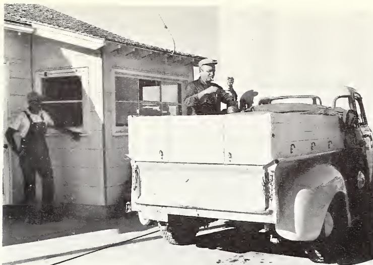
Figure 5. --Determining the test weight with portable test weight bucket and beam. Sideboards on pickup increase its capacity.
