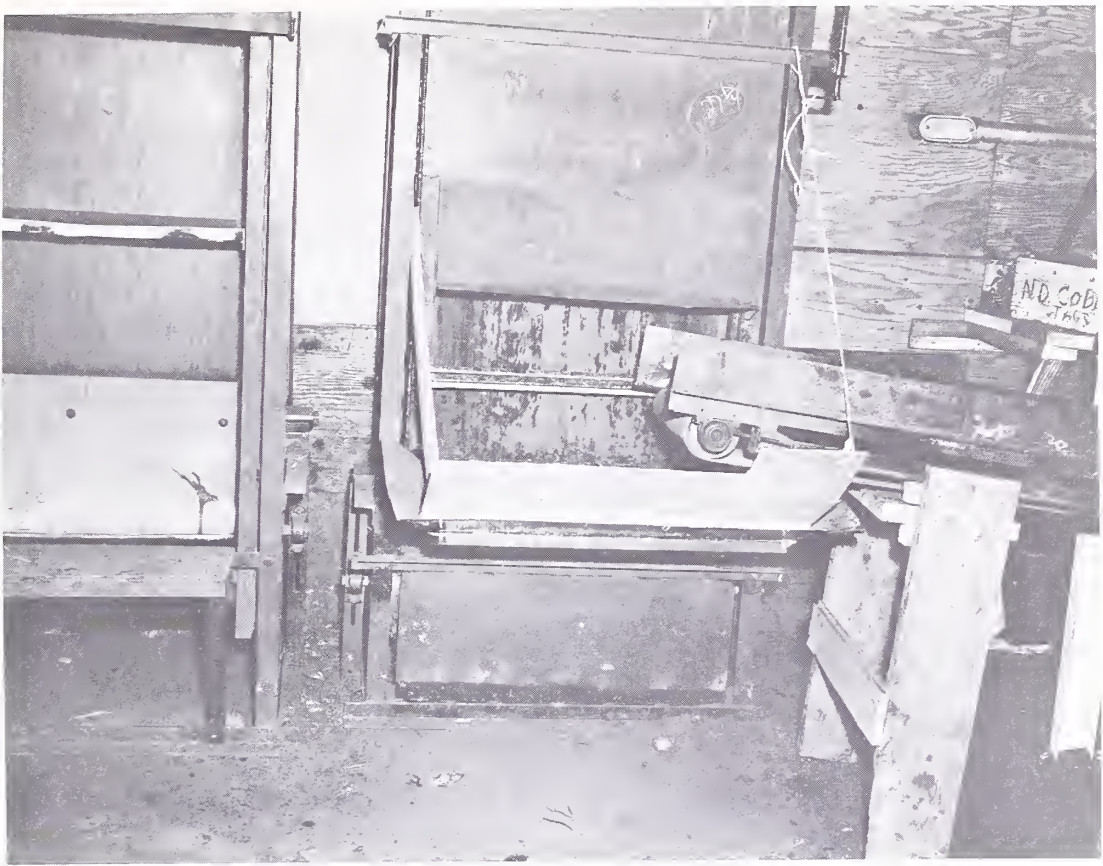
Figure 7.--Bulk bucket elevator (right) with flat-belt-conveyor extending into it; part of bag elevator is visible at left.
