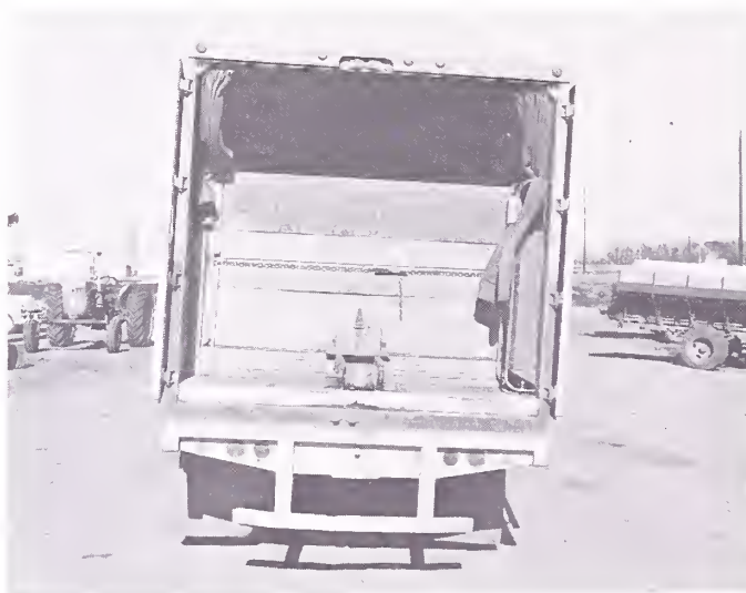
Figure 20.--Rear view of semitrailer (with tailgate doors open) in which a bulk bin is installed.
