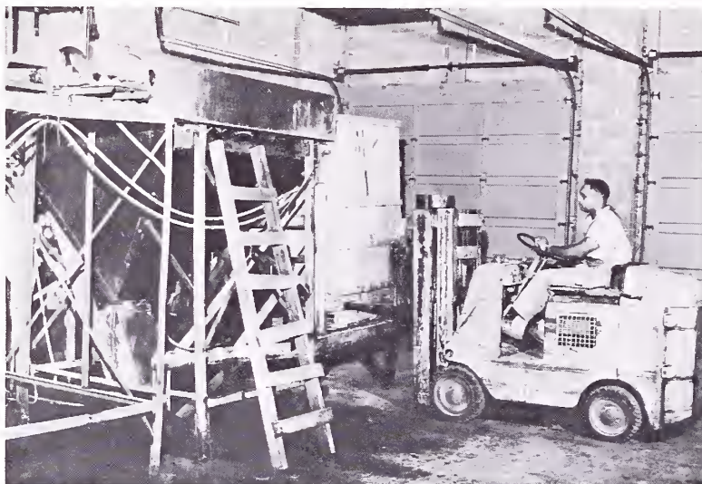
Figure 16.--Pallet box of potatoes being placed on the box tipper at the processing line.
