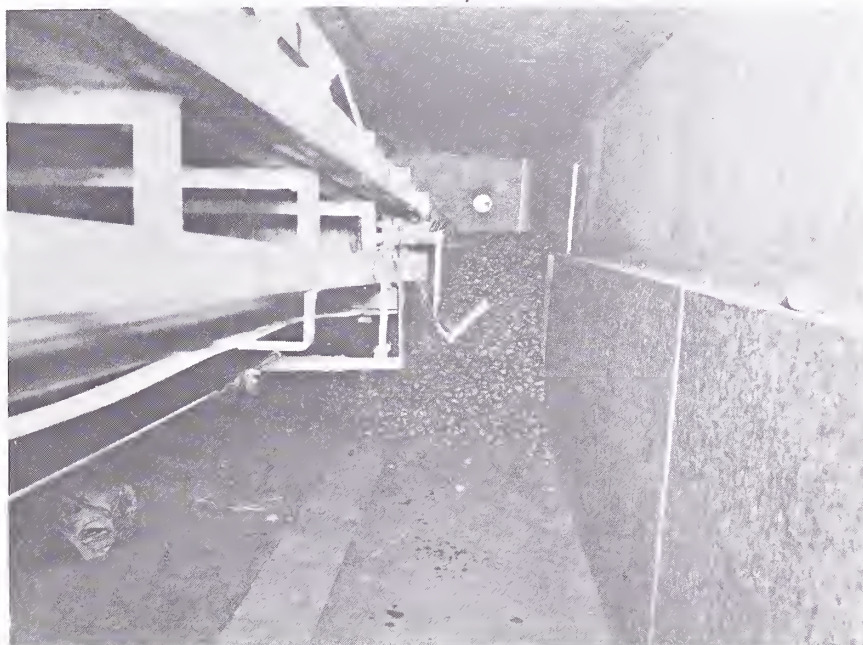
Figure 2.--Telescoping trough-belt conveyor, that moves potatoes into a truck, in telescoped and retracted position. Elevating cleated-belt conveyor is in side view at left.
