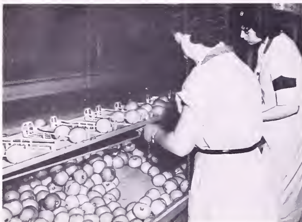
FIGURE 13.—In this method of packing, each worker places one or two tomatoes in the trays as they move past on the conveyor belt.
