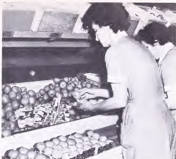
FIGURE 11.—After erecting tray by hand, packer selects and places one tomato at a time in the tray.
