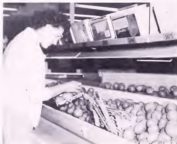
FIGURE 20.—Labor requirements were high for this one-hand tray-filling method.
