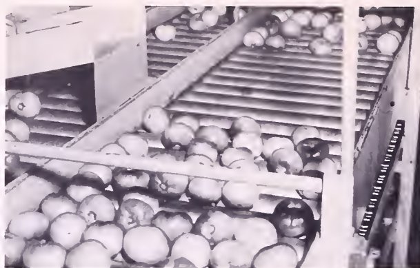
FIGURE 1.—Tomatoes are rotated and alined in rows as they move down this roller sorting table.
