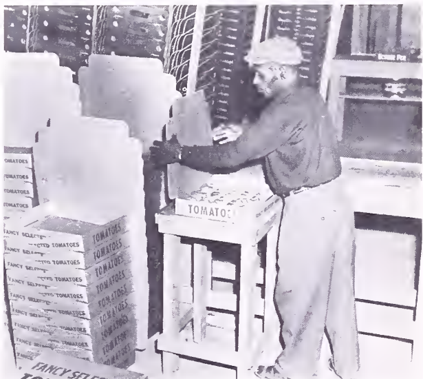
FIGURE 12.—This worker has placed 10 trays in a master container and is about to shape and close the hinge cover.
