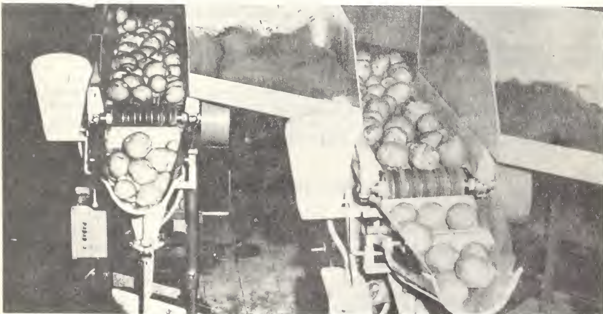
Figure 5.--Potatoes on conveyor flow into chutes leading to scales which are part of automatic bagging machine.
