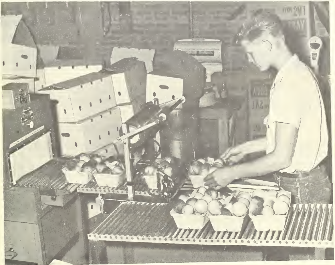
Figure 6.--Worker removes tills of peaches from conveyor and feeds them into machine which applies sleeve wrap of transparent film. (S.C. Agricultural Experiment Station photo.)
