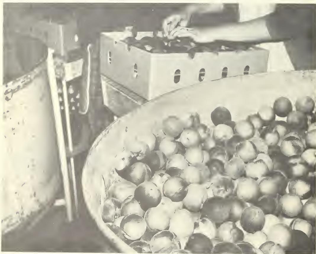
Figure 4.--A shipping tray in inner case of shallow fiberboard box is filled with sized peaches from tub. Note perforations in box, which will be matched by those in telescope cover to provide ventilation.
