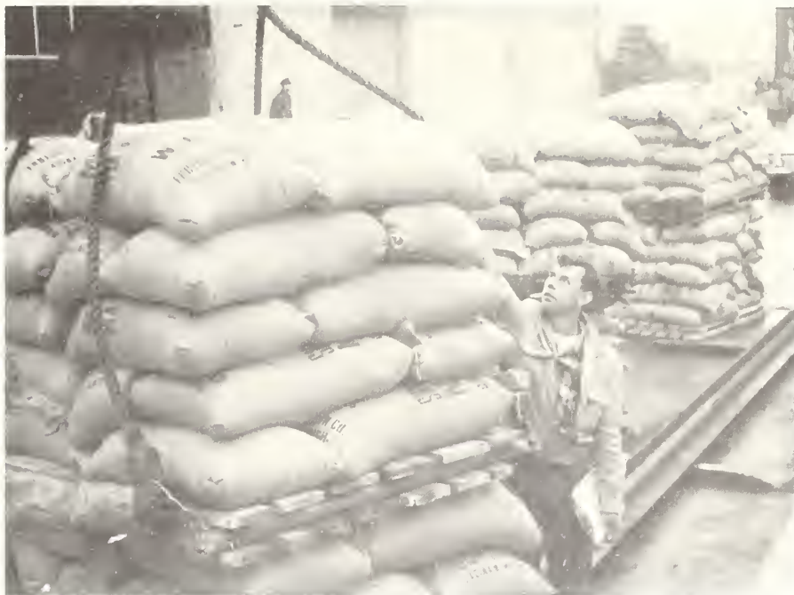
Figure 12. --Sampling procedure carried out at shipside from each pallet of 30 bags. A sample was taken from each pallet of 30 bags at shipside with a seed probe before beans were loaded onto the ship.
