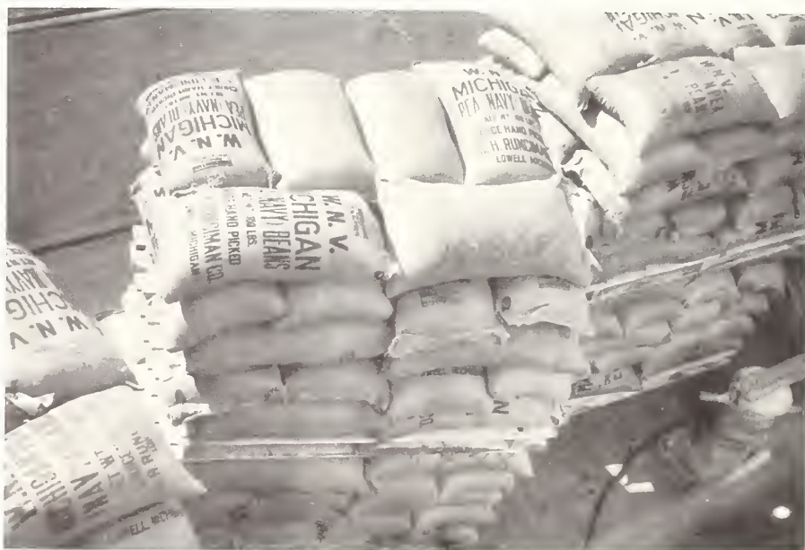
Figure 11. --Method of moving bagged beans to shipside on wooden pallets in the United States. Note how bags are interlocked to hold 30 containers on each pallet.
