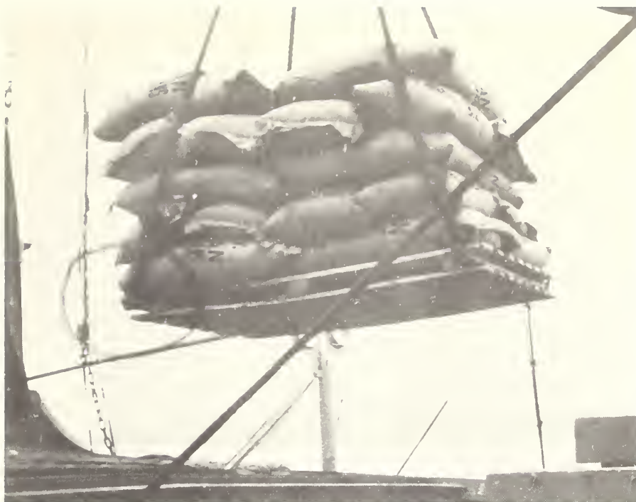
Figure 14. --This loaded pallet is being lowered into the hold. Two bags on upper left and the line at lower left (circled) have begun to slip. Often, several bags are broken when a rope slips off a pallet.
