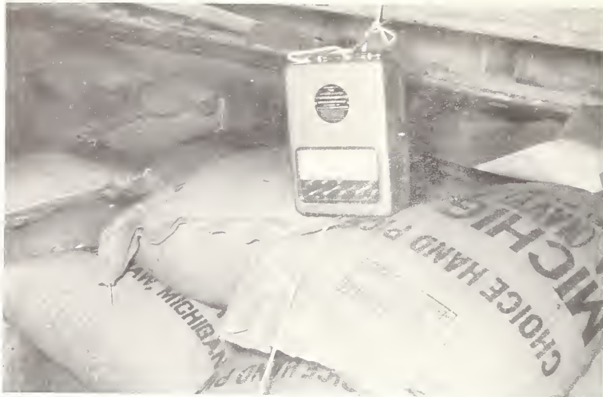
Figure 10. --A hygromograph with 24-hour chart was placed over the commodity and under the ship's deck to measure temperature and humidity at this point.
