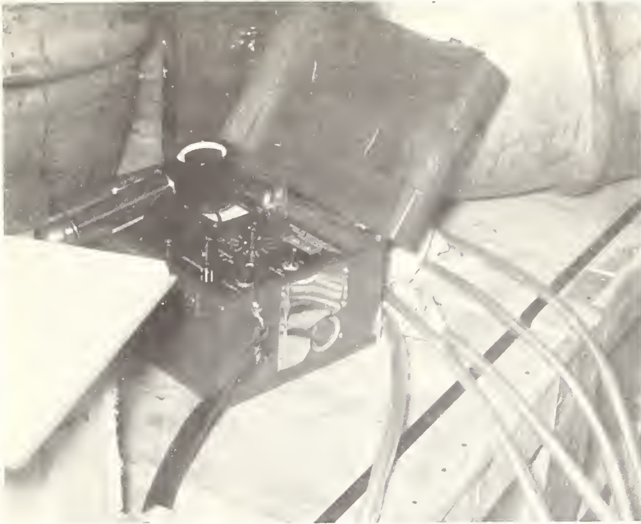
Figure 6. --The leads for the 5 cables were arranged so that temperatures from all 60 points could be read from this one instrument.
