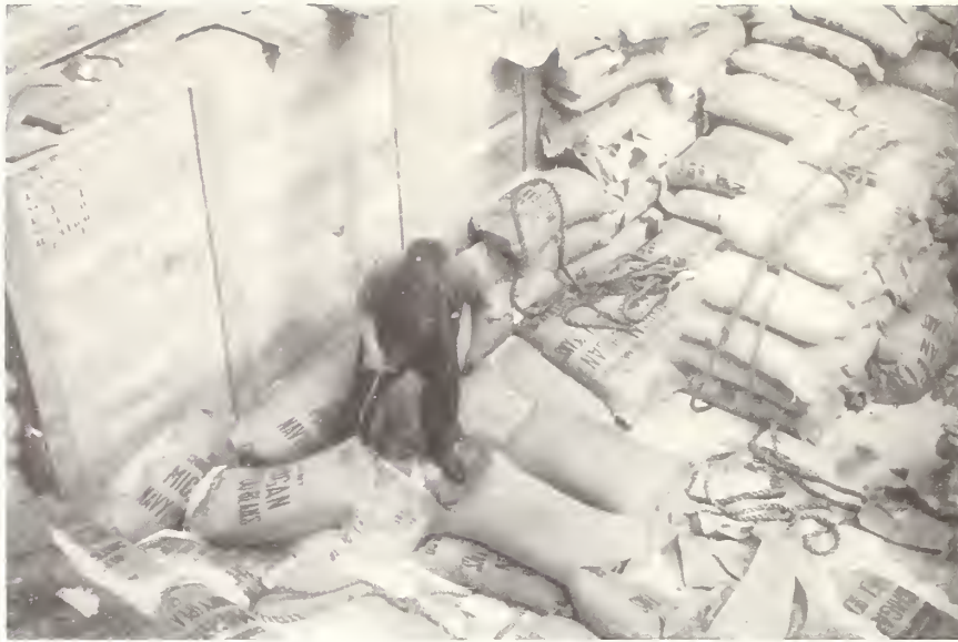
Figure 30. --Rough dunnage, corners of large crates, and cargo hooks cause many broken bags during unloading. Loose beans are scattered over load.
