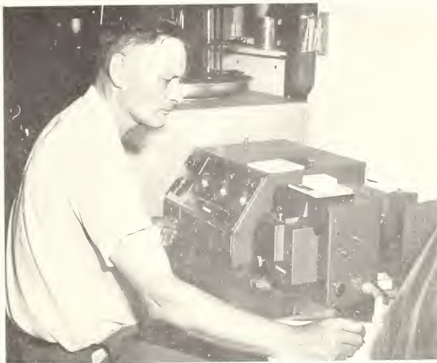
Figure 9. --A color difference meter was used in determining the amount of color change in overseas shipment of beans.
