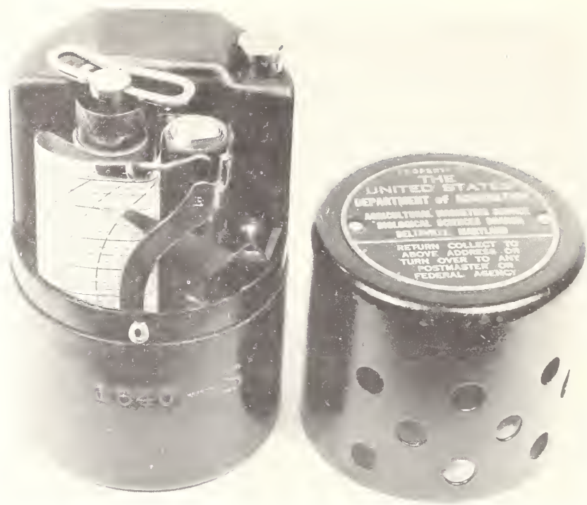
Figure 7. --Recording thermometers were used in two of the shipments. These thermometers are used extensively in test shipments of fruits, vegetables, and other produce.
