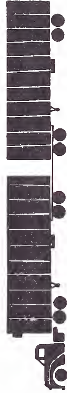
9-Axle Tractor, Semitrailer and Full Trailer Combination
