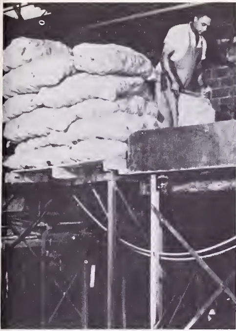
Figure 6.--Emptying bags into the hopper.
