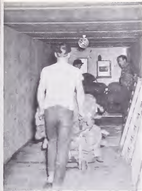
Figure 2.--Handtrucking and stowing bags in the truck.
