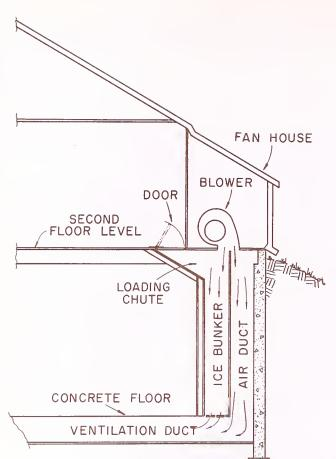
Figure 5.--Installation of the ice bunker, shown at left, in the ice refrigerated storage provided for a portion of the ventilating air to flow across the surface of the ice for cooling (used in Storage No. 4).
