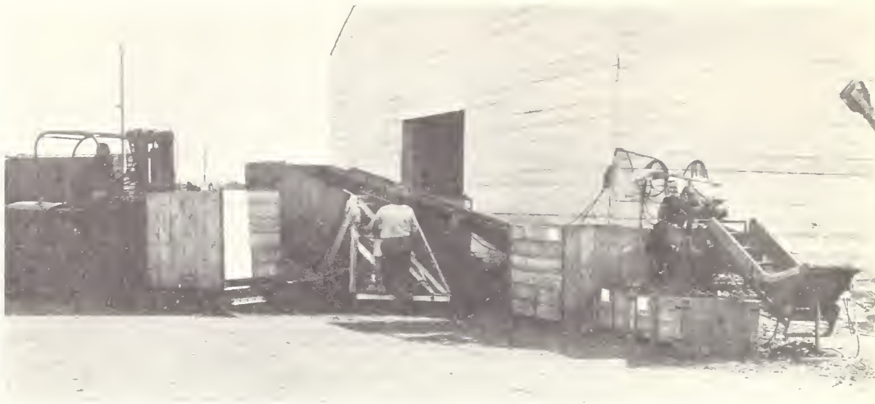
FIGURE 15.—Draper chain conveyor, sizer and sorting table; trough belt conveyor; box tipper; roller conveyor; and forklift truck (from right to left).
