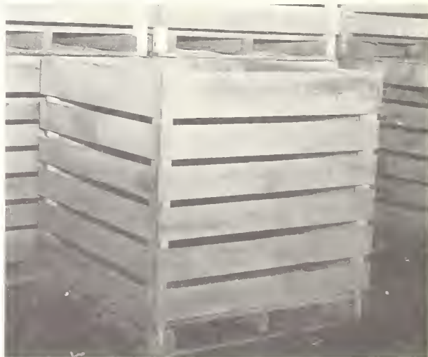
FIGURE 17.—A 1-ton capacity pallet box with spaced sides and bottom.
