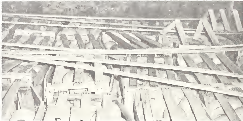
Figure 2.--Cross section of a partly unloaded shipment of cantaloups in conventional jumbo crates showing container breakage in load at one end of car.
