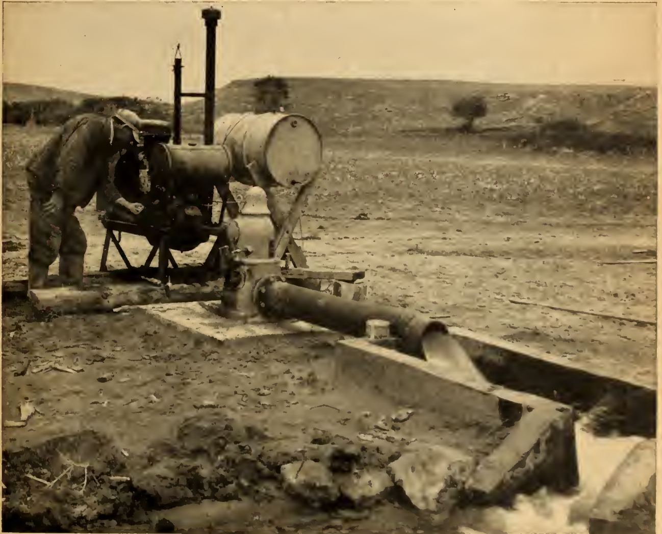
Modern pumps make irrigation cheaper and easier. This one in the Republican Valley, Nebr., delivers 750 gallons of water a minute.
