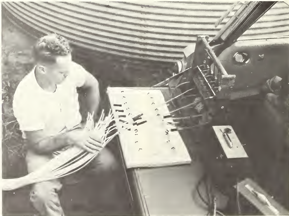
FIGURE 3.—Glass collection tubes and purging apparatus used to trap fumigant samples for gas chromatography analyses.
