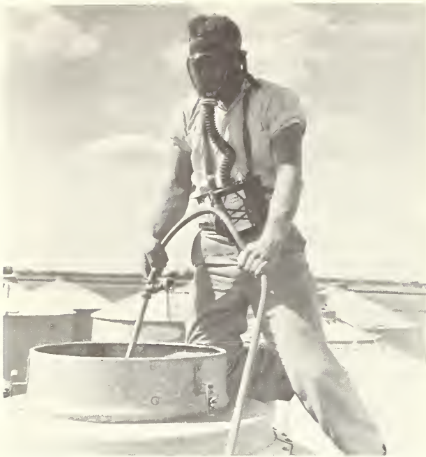
FIGURE 2.—Application of liquid fumigants through roof opening using a hand-held nozzle.
