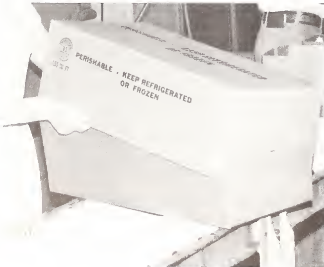
Figure 4.—A full-telescoping fiberboard box for bagged poultry.
