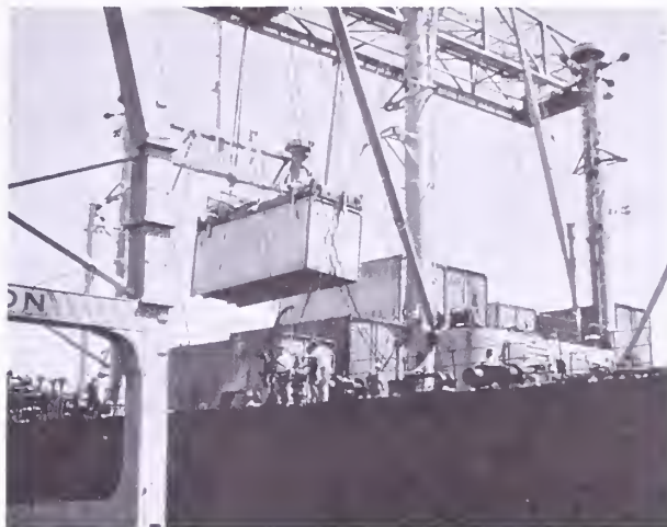
FIGURE 11.—Container being loaded aboard container-ship by shoreside gantry crane.
