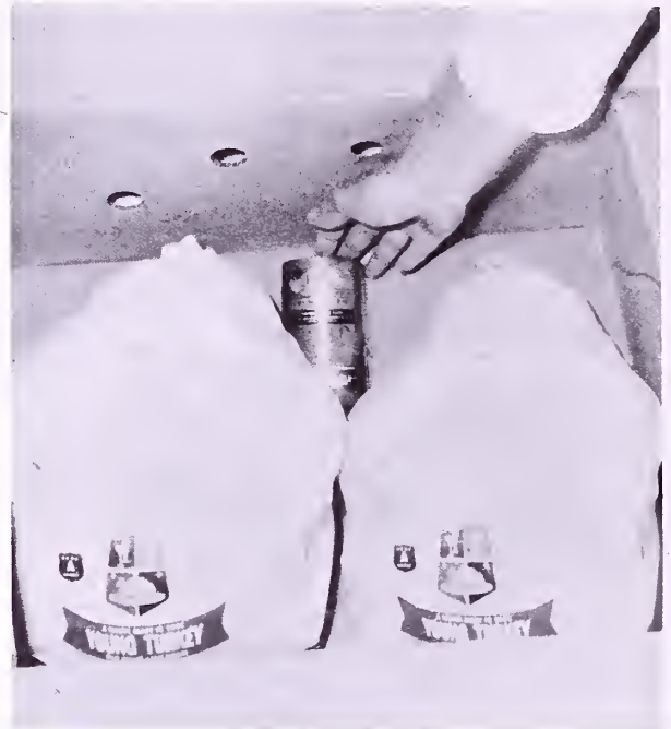
FIGURE 1.—Placing recording thermometer in poultry box when loading at poultry plant.
