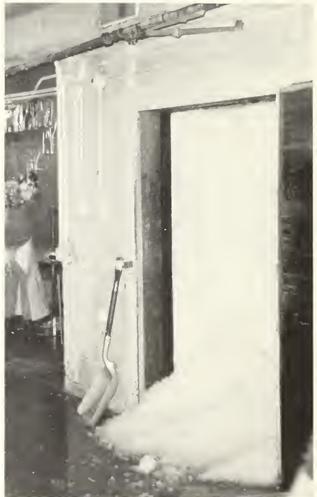
Figure 5. —Ice is discharged onto floor of packing area when door of ice-storage bin is opened.
