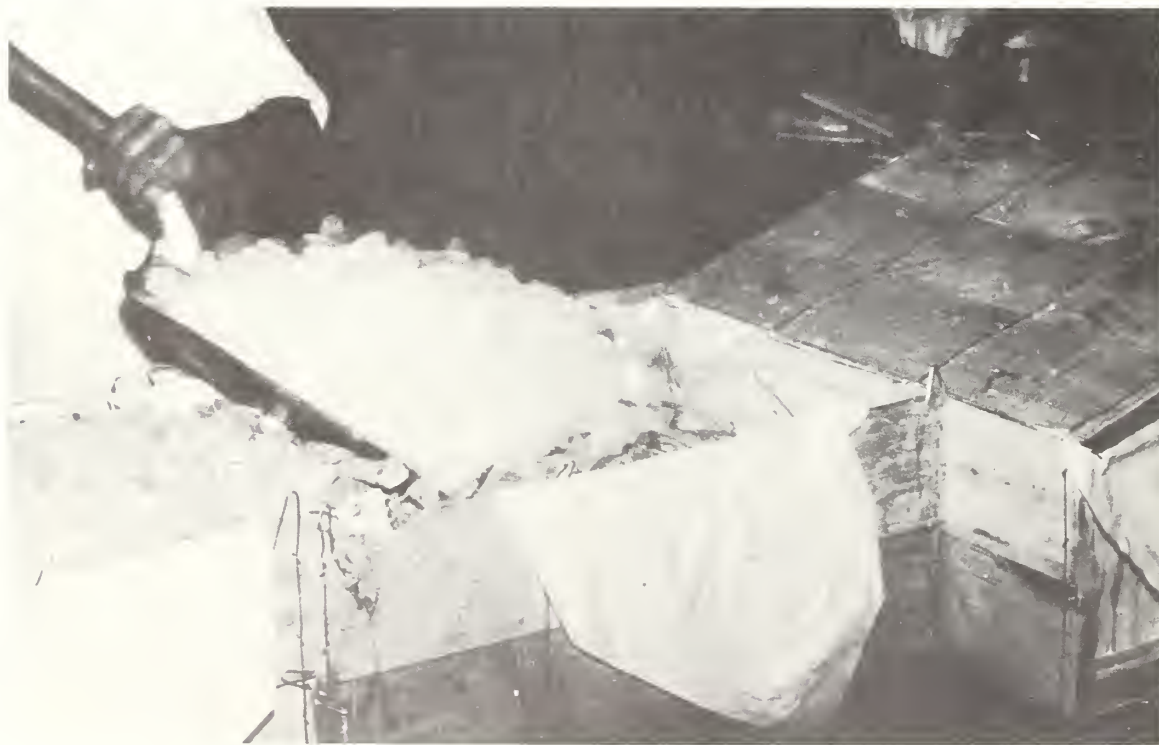
FIGURE 1.—Conventional wirebound wood-vener box packed with poultry and ice. Note paper liner.
