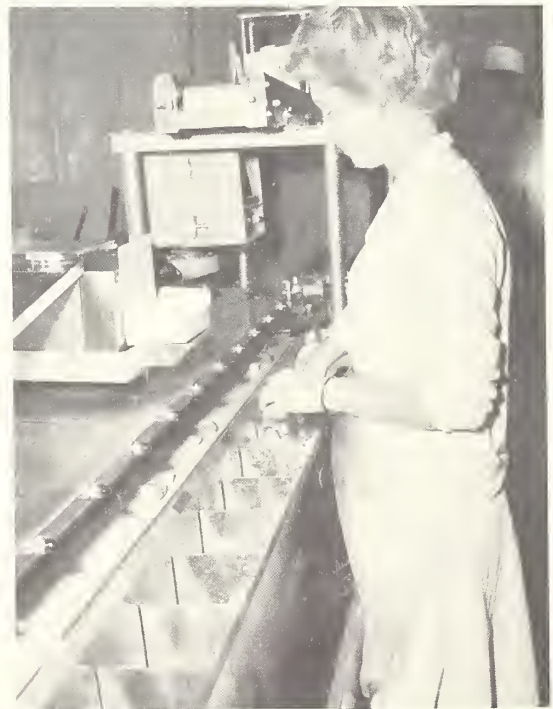
FIGURE 4.—Operator at packing station in front of checkweigher scale and packing platform.
