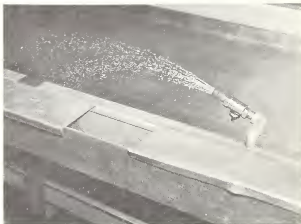
FIGURE 27.—An improved trim station for the heart and liver operation. A spray nozzle and funnel to giblet flume are attached to the side of the offal trough to reduce worker reach and encourage frequent hand rinse.
