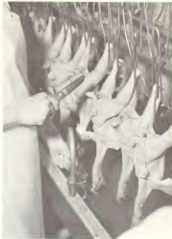
FIGURE 68.—Rinsing the hand with the gooseneck type, open-pipe nozzle.
