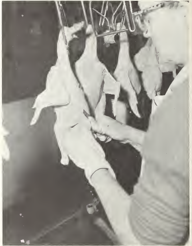
FIGURE 9.—Removing preen gland with bird suspended by the neck.
