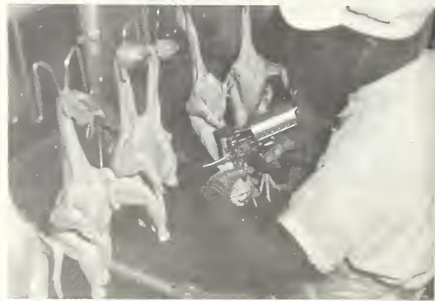
FIGURE 6.—Mechanized shears used to remove shanks.
