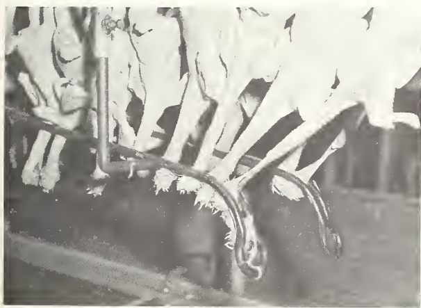
FIGURE 48.—A stationary head puller removing heads from eviscerated poultry.
