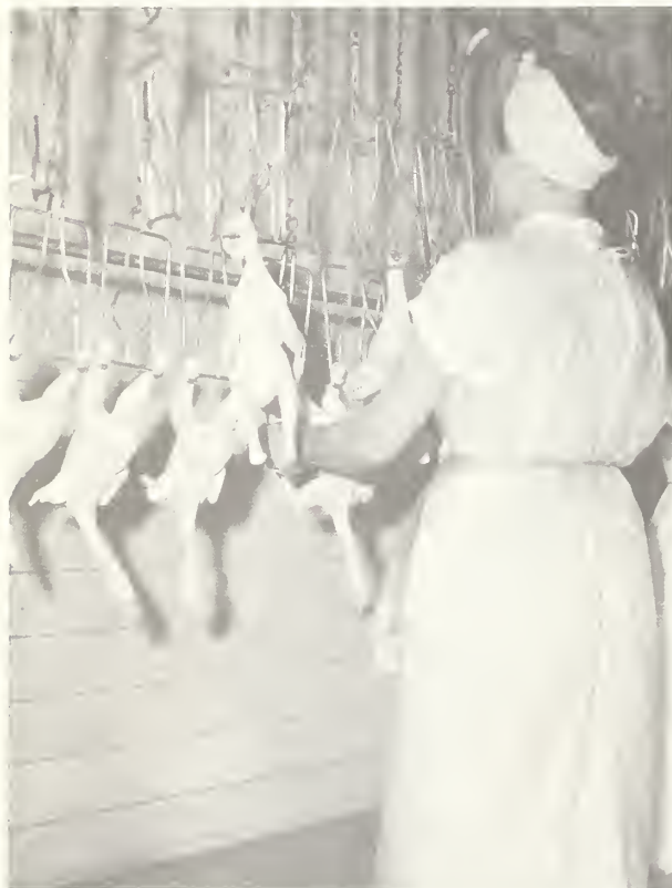
FIGURE 10.—Transferring poultry directly from the picking line to the eviscerating line using the neck-to-hock method. The picking line path is the high line close to the operator.
