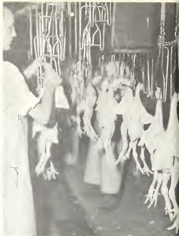
FIGURE 11.—Transferring poultry from the defeathering line to the eviscerating line using direct neck-to-neck method.
