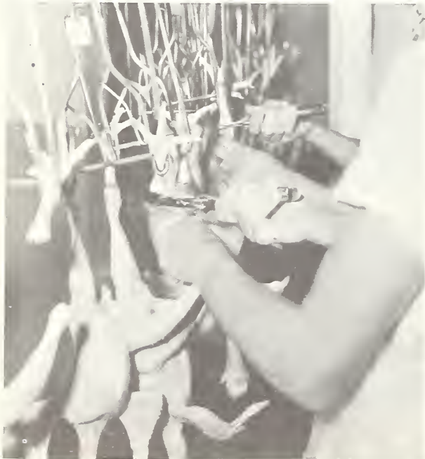
FIGURE 5.—Removing chicken shanks with manual shears.
