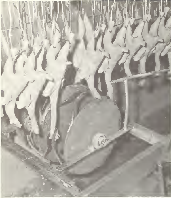
FIGURE 49.—A rotating drum-type head puller mounted on eviscerating line.
