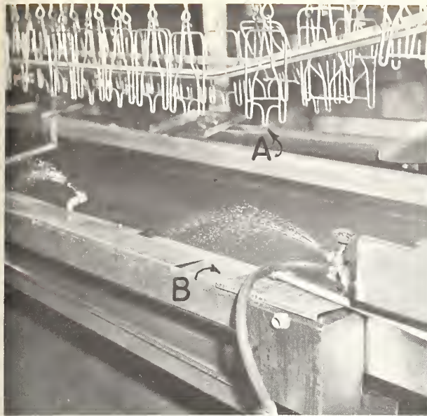
FIGURE 62.—An improved heart and liver trim station. The water spray is in the path of the worker's hands as they move from point of removal (A) to flume opening (B).
