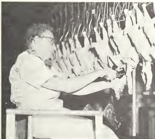
FIGURE 57.—One operator cutting necks from birds on two eviscerating lines which are routed close together. Neck vertebrae have been snipped and operator is using a knife to cut through remaining neck skin.
