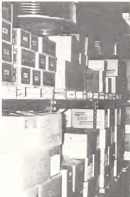
FIGURE 10.—Pallet racks for less than full pallet loads conserve cooler space.
