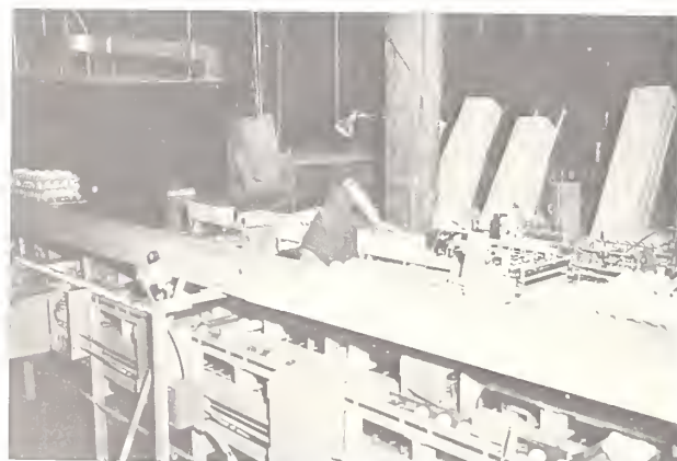
FIGURE 41.—Column interference can affect layout efficiency and servicing schedules.
