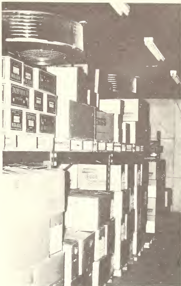
FIGURE 33.—Pallet racks help conserve cooler floorspace because pallet loads that are of less than maximum size can be stacked one over the other.
