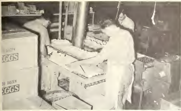
FIGURE 14a.—The advantages of increased production of this mechanized egg grading and packing line are largely offset by rehandling required in crowded area.
