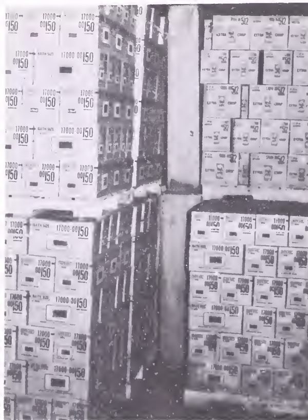
FIGURE 4.—Box-type bumpers between pallet loads in center of railcar. Note banding on top layer of each pallet load.
