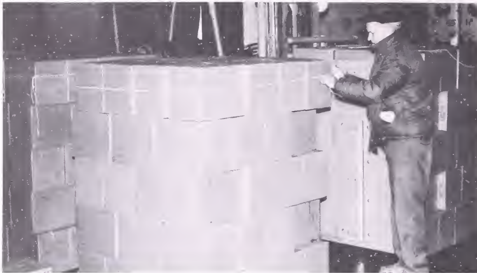
FIGURE 3.—Securing top layer of a pallet unit load with heavy string.
