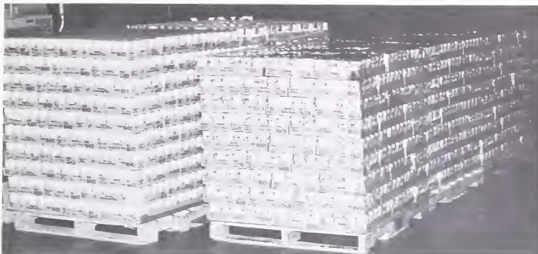
FIGURE 8.—Individual tray pack cases wrapped with shrink film on pallets.
